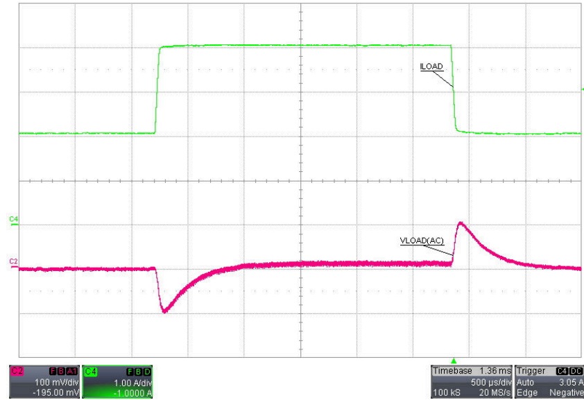
Figure 4-15. Load Transient, V_{SUPPLY} = 36\text{ V} , I_{LOAD} = 2\text{ A to }4\text{ A}
