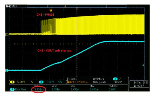
Figure 7-13. PVIN=12 V, VOUT=3.3 V, IOUT= 6 A, FSW=500 kHz: Soft Start
