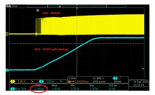
Figure 7-6. PVIN=5 V, VOUT=1.8 V, IOUT=6 A, FSW=500 kHz: Soft Start
