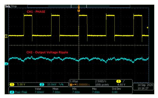
Figure 7-12. PVIN=12 V, VOUT=3.3 V, IOUT= 6 A, FSW=500 kHz: Output Voltage Ripple
