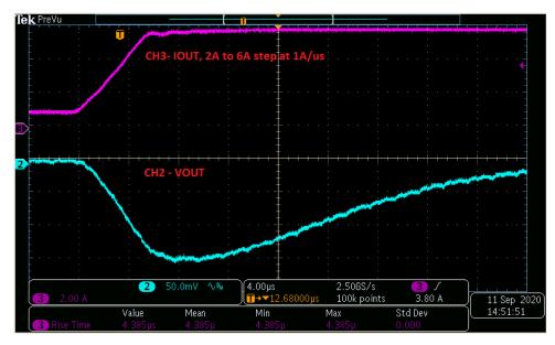
Figure 7-10. PVIN=12 V, VOUT=3.3 V, FSW=500 kHz: Transient Response to current step from 2 A to 6 A at 1 A/us
