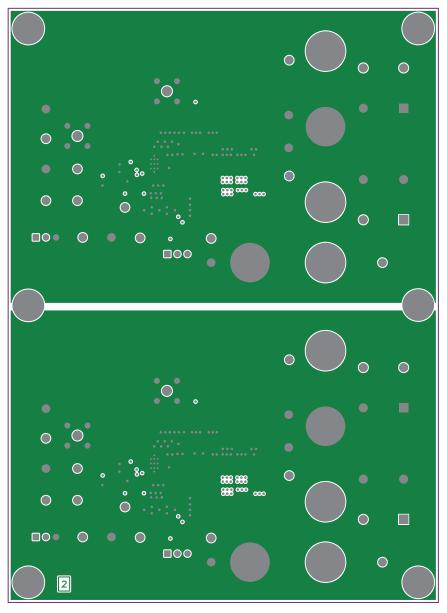
Figure 5-3. Mid-Layer 1 Ground Plane
