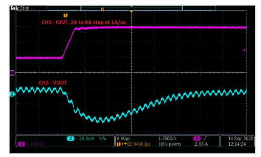
Figure 7-3. PVIN=5 V, VOUT=1.8 V, FSW=500 kHz: Transient Response to current step from 2 A to 6 A at 1 A/us
