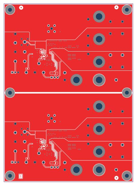
Figure 5-2. Top Layer Routing
