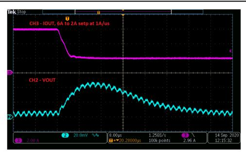
Figure 7-4. PVIN=5 V, VOUT=1.8 V, FSW=500 kHz: Transient Response to current step from 6 A to 2 A at 1 A/us
