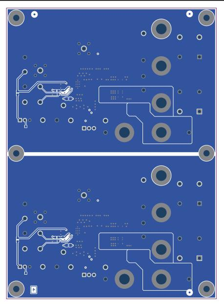
Figure 5-5. Bottom Layer Routing
