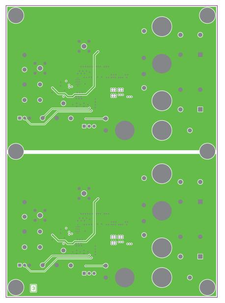
Figure 5-4. Mid-Layer 2 Routing
