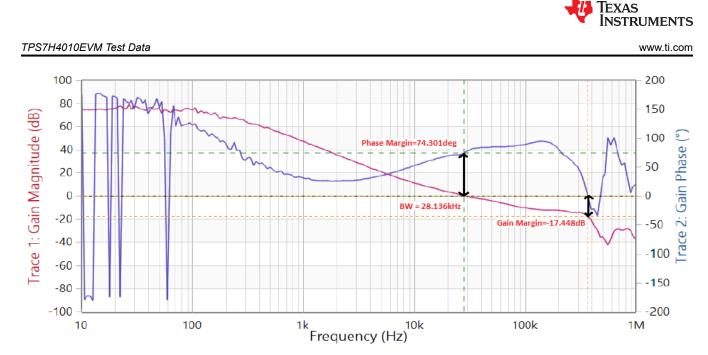
Figure 7-2. PVIN=5 V, VOUT=1.8 V, IOUT=6 A, FSW=500 kHz: Loop Response
