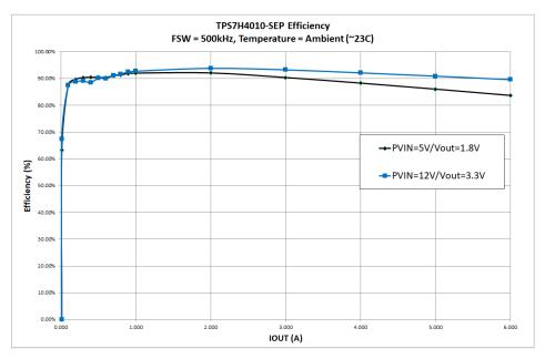
Figure 7-7. FSW=500 kHz: Efficiency vs IOUT
