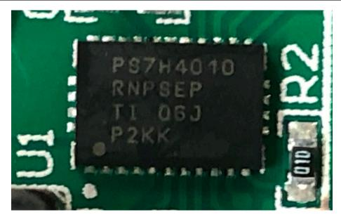
Figure 1-4. TPS7H4010-SEP Package Marking
