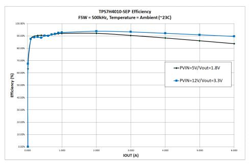
Figure 7-14. FSW=500 kHz: Efficiency vs IOUT
