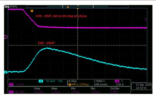
Figure 7-11. PVIN=12 V, VOUT=3.3 V, FSW=500 kHz: Transient Response to current step from 6 A to 2 A at 1 A/us
