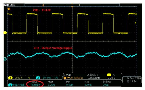
Figure 7-5. PVIN=5 V, VOUT=1.8 V, IOUT=6 A, FSW=500 kHz: Output Voltage Ripple
