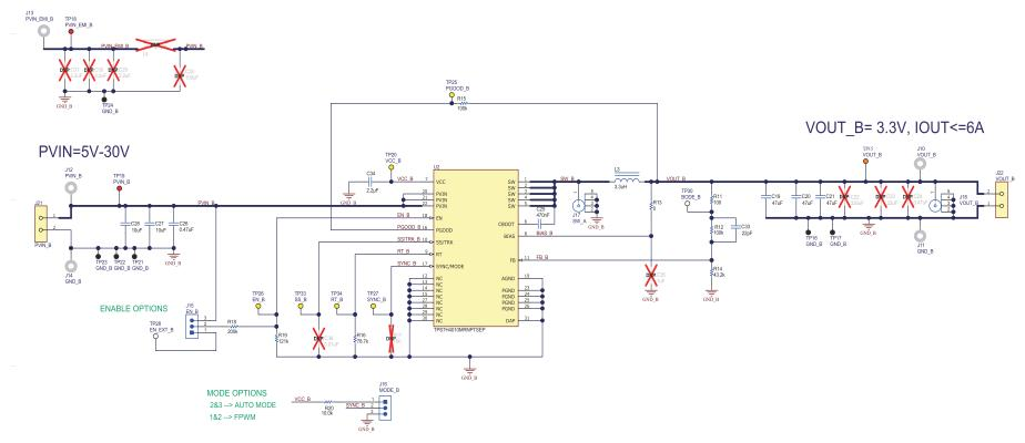
Figure 4-2. TPS7H4010EVM PVIN=12 V, VOUT=3.3 V Schematic
