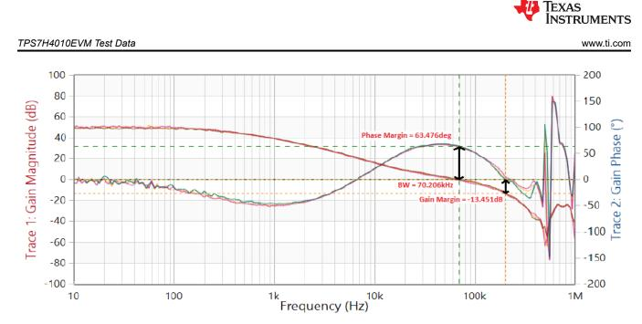
Figure 7-9. PVIN=12 V, VOUT=3.3 V, IOUT=6 A, 3 A, 1 A, FSW=500 kHz: Loop Response
