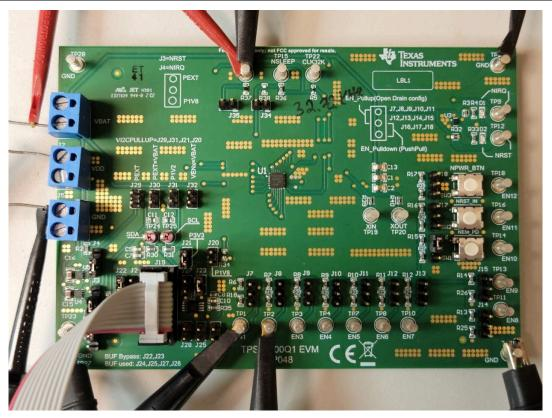
Figure 4-1. EVM Connections for Testing EN1 and EN2
