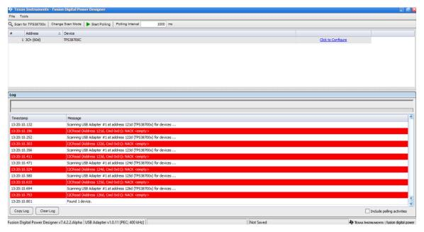
Figure 4-19. Fusion Scan Window - Scan for TPS38700Q1EVM Completed
