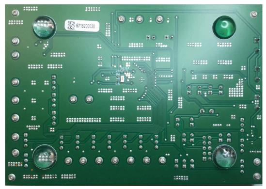
Figure 1-2. TPS38700Q1EVM Board Bottom
