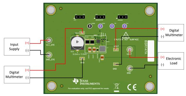
Figure 1-1. EVM Board Connections
