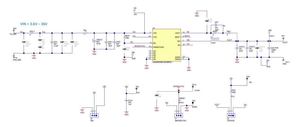
Figure 3-1. LMQ66430-2EVM Schematic
