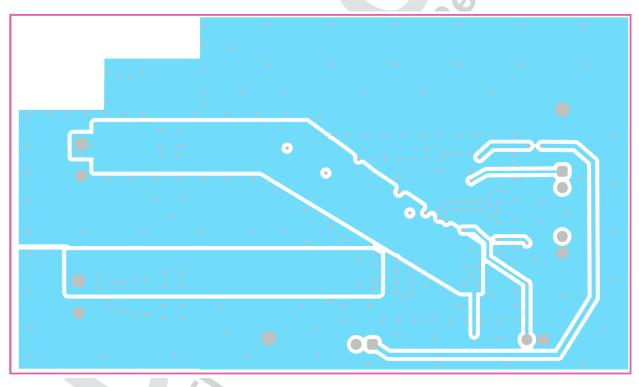
Figure 4-3. Mid-Layer 2 Routing
