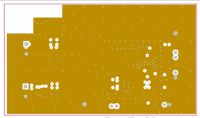
Figure 4-2. Mid-Layer 1 Ground Plane
