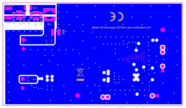
Figure 4-4. Bottom Layer Routing
