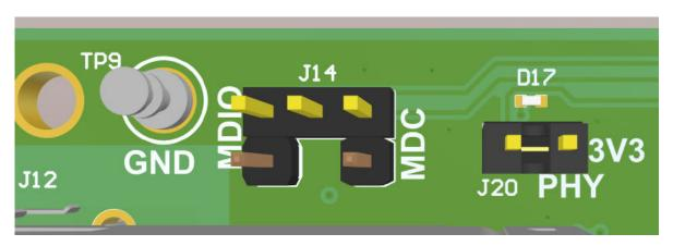
Figure 2-5. Onboard MSP Connections for MDIO and MDC
