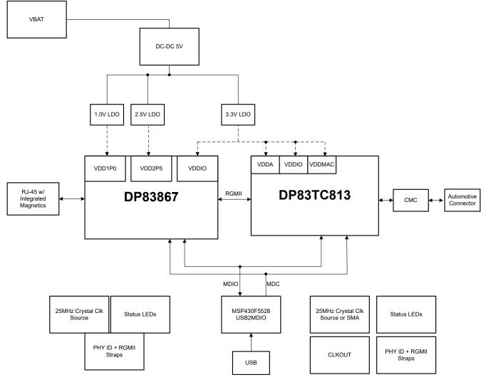
Figure 3-1. DP83TC813EVM-MC Block Diagram
