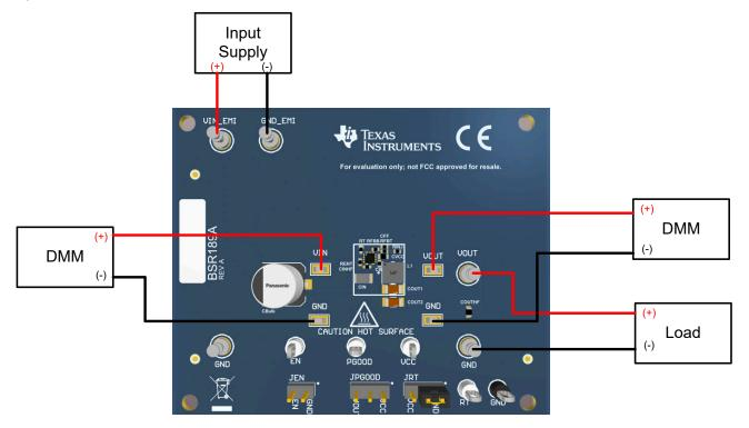
Figure 1-1. EVM Board Connections
