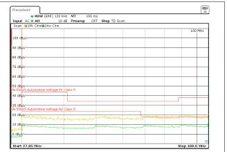
Figure 6-13. LMR43620RQ5EVM-400 High Frequency Conducted EMI Results 12.5  $V_{IN}$ , 5  $V_{OUT}$ ,  $I_{OUT}$  = 2 A (Green-Average Scan and Yellow-Peak Scan)
