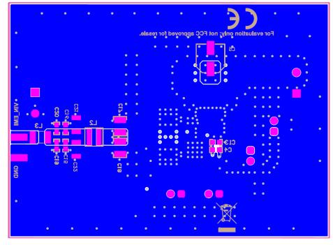
Figure 5-4. Bottom Layer Routing
