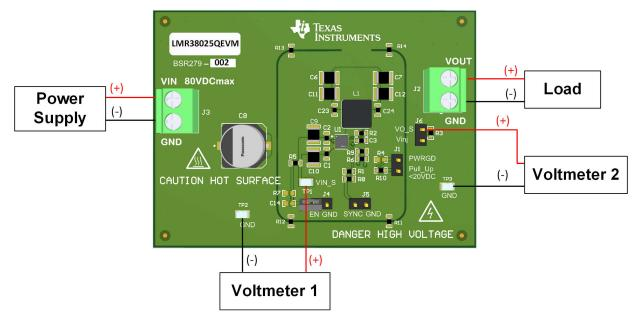
Figure 2-1. LMR38025Q EVM Setup
