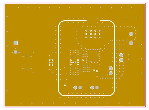
Figure 5-2. Mid-Layer 1 Ground Plane
