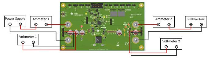
Figure 3-1. Typical EVM Connection Diagram
