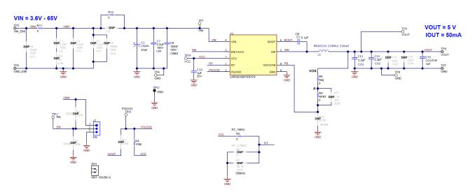
Figure 4-1. LMR36500EVM Schematic
