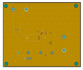
Figure 4-3. PCB Ground Layer (Directly below top layer)
