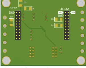
Figure 4-3. Component Placement - Bottom Assembly
