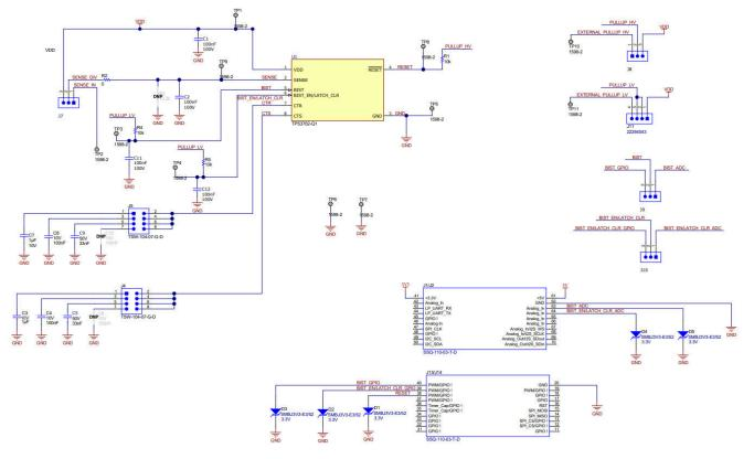
Figure 4-1. TPS376XEVM Schematic
