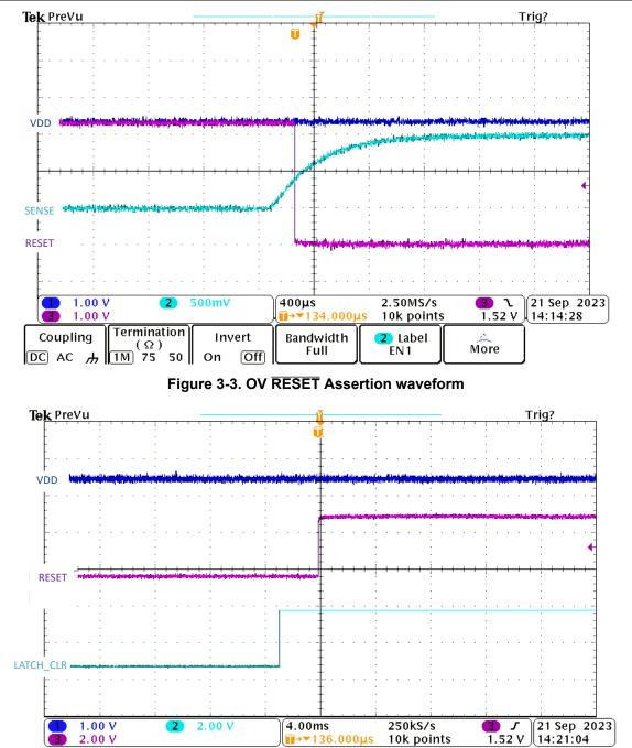
Figure 3-4. RESET Unlatch waveform
