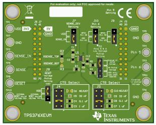
Figure 4-2. Component Placement - Top Assembly
