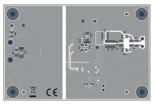
Figure 4-7. Bottom Layer Silkscreen (Bottom View)
