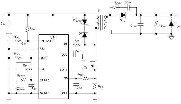
Figure 1-1. LM5185 PSR Flyback Converter Simplified Schematic
