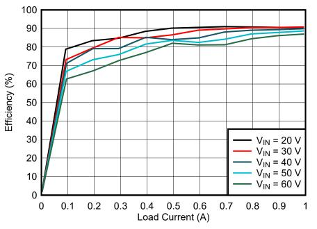
Figure 3-1. EVM Efficiency vs. Load and Input Voltage
