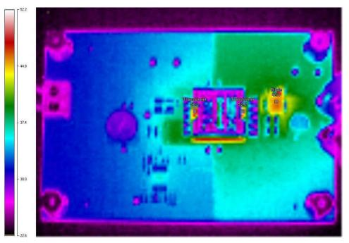
Figure 3-9. EVM Thermal Image. Vin=48V, lout=1.0A
