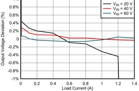
Figure 3-2. EVM Output Voltage Regulation vs Load and Input Voltage
