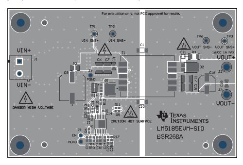
Figure 4-2. Top Layer Silkscreen (Top View)
