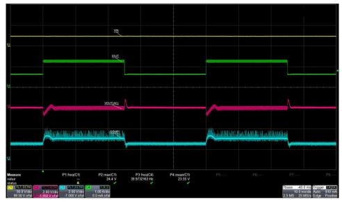
C1=Vin; C2=Vout (ac coupled); C3=Vcomp; C4=Iout
