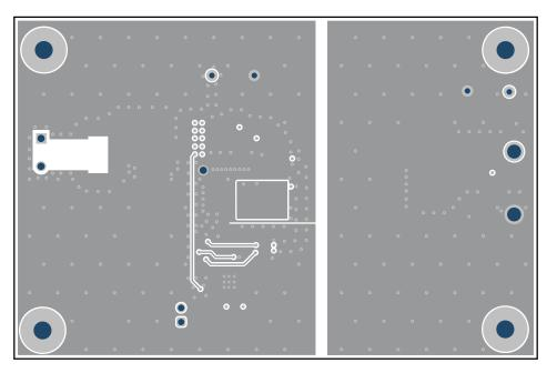
Figure 4-5. Mid Layer 2 Layout (Top View)
