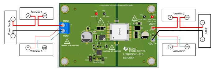
Figure 2-1. EVM Test Setup
