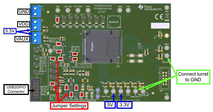
Figure 2-4. TPS389C0XEVM Monitoring Two Voltage Supply Rails
