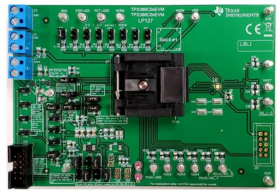
Figure 2-1. TPS389C0XEVM Board Front
