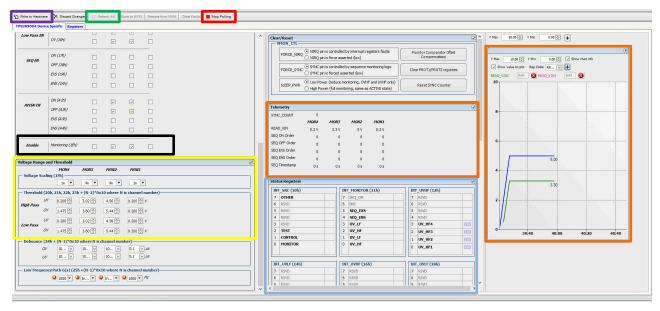
Figure 2-5. TPS389C0XEVM GUI Setup for Monitoring Two Voltage Supply Rails
