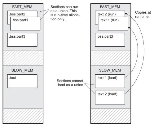
Figure 8-4. Memory Allocation Shown in Example 8-13 and Example 8-14
