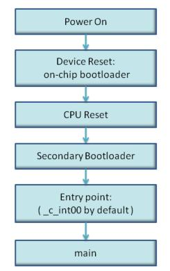
Figure 3-2. Bootloading Sequence with Secondary Bootloader
