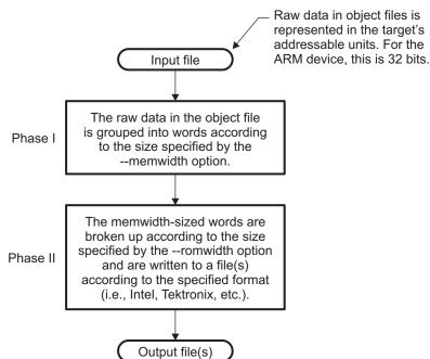
Figure 12-2. Hex Conversion Utility Process Flow
