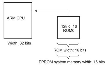
For this scenario, the application code and data reside on the EPROM: the lower 64K words of EPROM memory are dedicated to application code space and the upper 64K words are dedicated to the data tables. The application code is loaded starting at address 0x0 on the EPROM but maps to the TMS470 CPU at address 0x3000. The data tables are loaded starting at address 0x1000 on the EPROM and map to the TMS470 CPU address 0x20.
