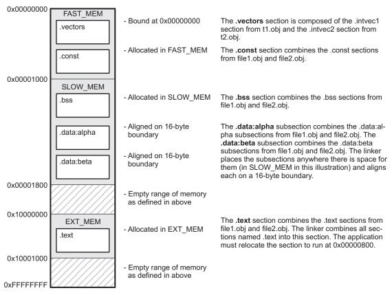
Figure 8-2. Section Placement Defined by Example 8-5
