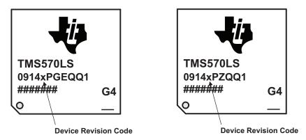
Figure 1. Device Revision Code Identification
