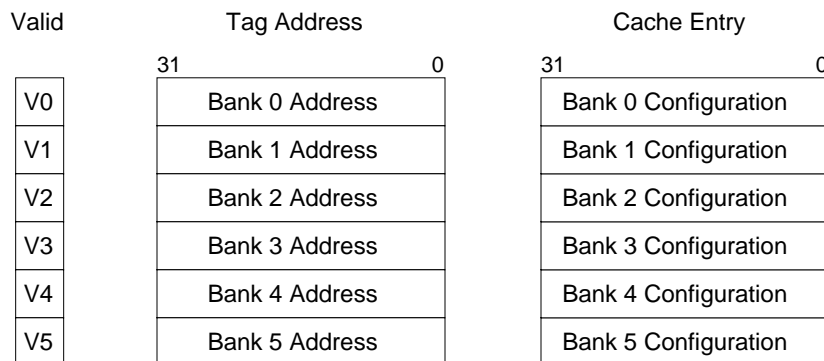
Figure 10–2. Cycle Configuration Cache Structure
