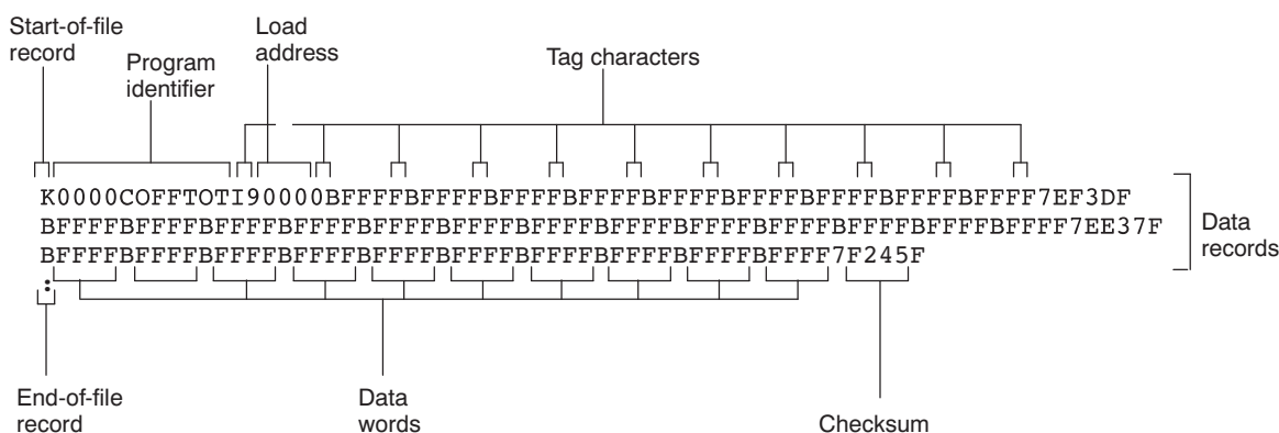
Figure 12-13. TI-Tagged Object Format
