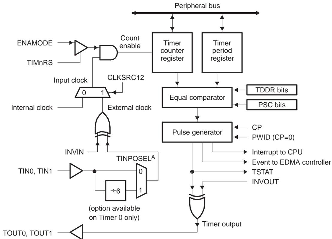
A These options are set in the timer control register (TIMERCTL) within the System Module.
