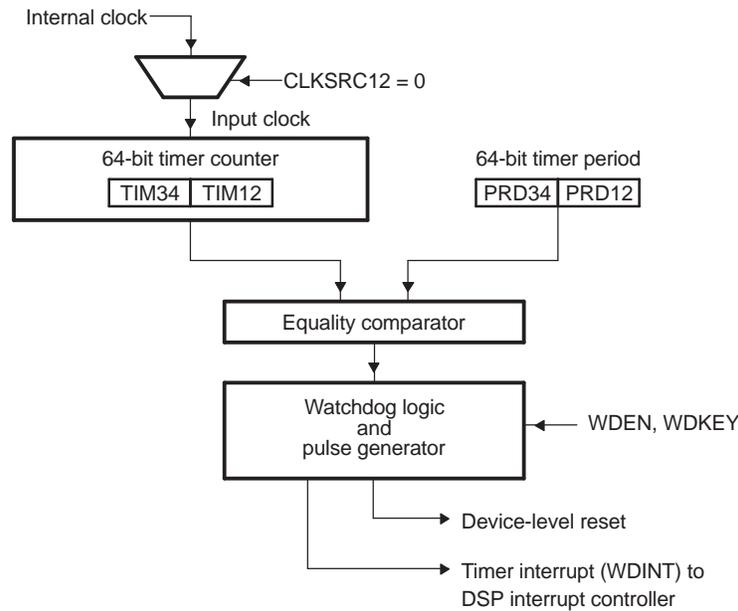
Figure 10. Watchdog Timer Operation State Diagram
