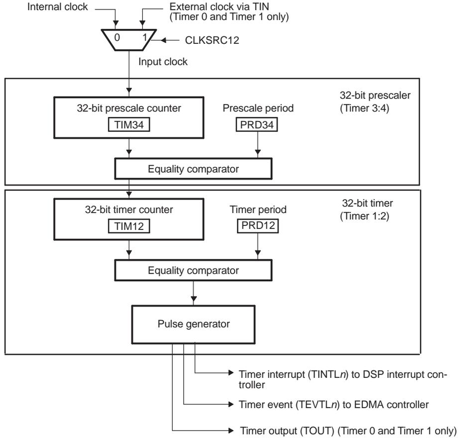
**Figure 5. Dual 32-Bit Timers Chained Mode Example**
