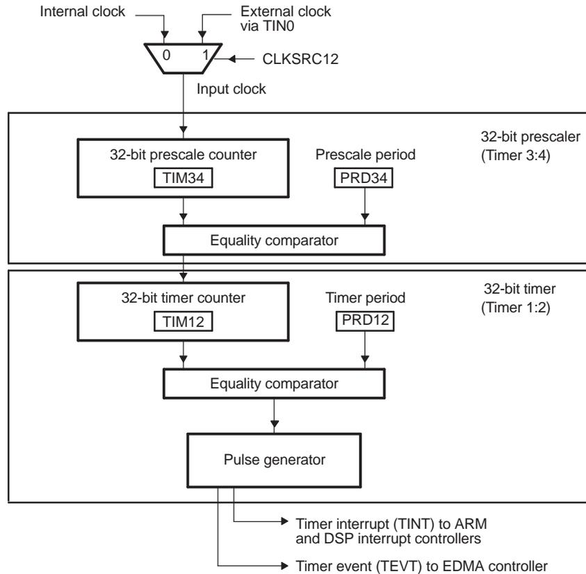
**Figure 5. Dual 32-Bit Timers Chained Mode Example**
