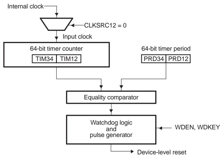
Figure 10. Watchdog Timer Operation State Diagram
