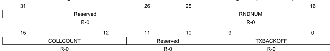
Figure 75. Back Off Random Number Generator Test Register (BOFFTEST)
