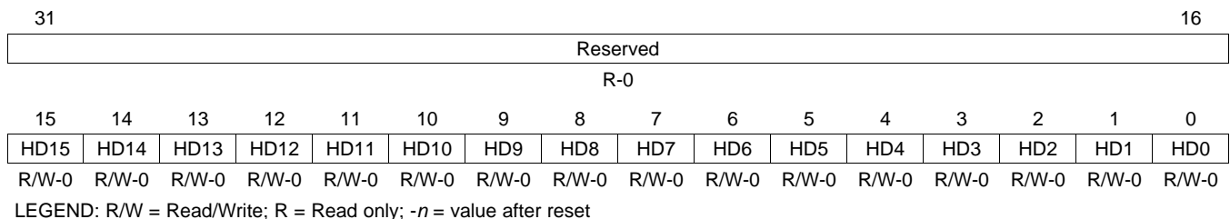
Figure 21. GPIO Data 1 Register (GPIO_DAT1)
