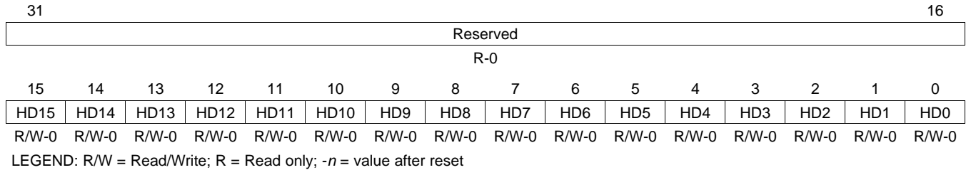
Figure 20. GPIO Direction 1 Register (GPIO_DIR1)
