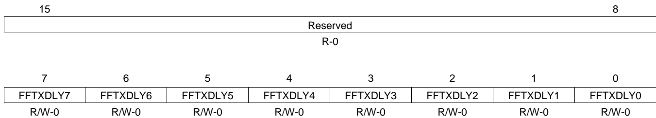
Figure 2-11. SPI FIFO Control (SPIFFCT) Register – Address 704Ch
