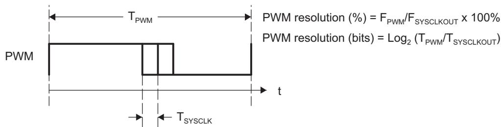
If the required PWM operating frequency does not offer sufficient resolution in PWM mode, you may want to consider HRPWM. As an example of improved performance offered by HRPWM, [Table 1](#) shows resolution in bits for various PWM frequencies. These values assume a MEP step size of 60 ps. See the device-specific datasheet for typical and maximum performance specifications for the MEP.
