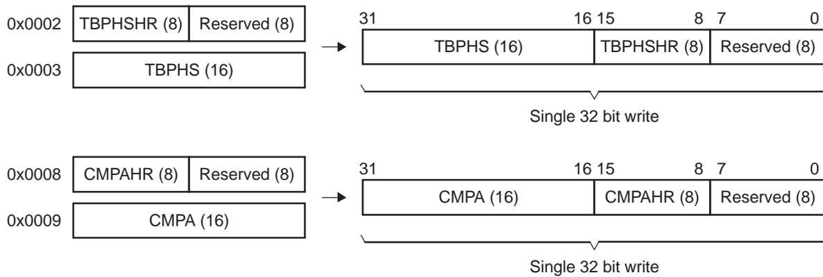
HRPWM capabilities are controlled using the Channel A PWM signal path. Figure 4 shows how the HRPWM interfaces with the 8-bit extension registers.
