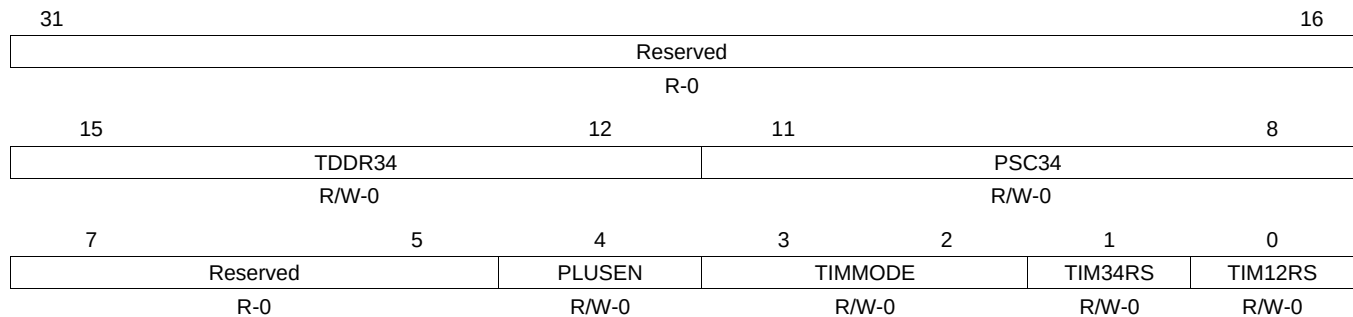
Figure 30-22. Timer Global Control Register (TGCR)
