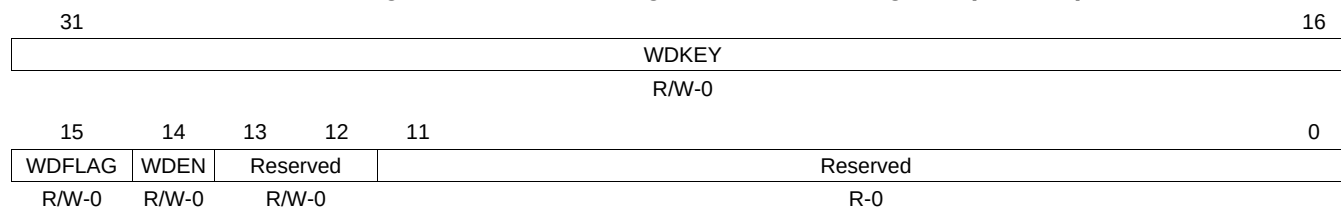
Figure 30-23. Watchdog Timer Control Register (WDTCR)
