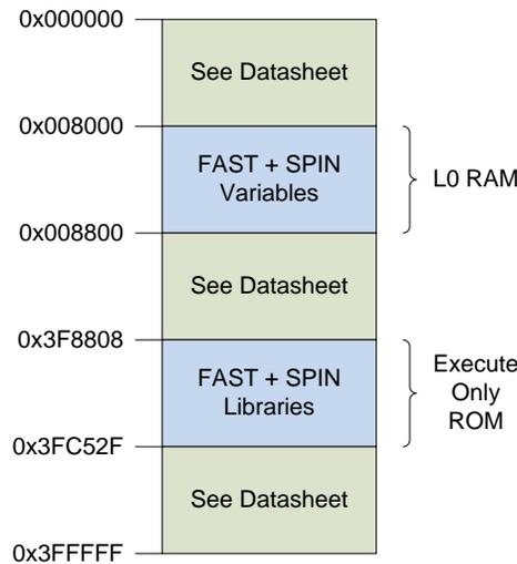
**Figure 8. F2805xF Allocated Memory for InstaSPIN-FOC Library**
