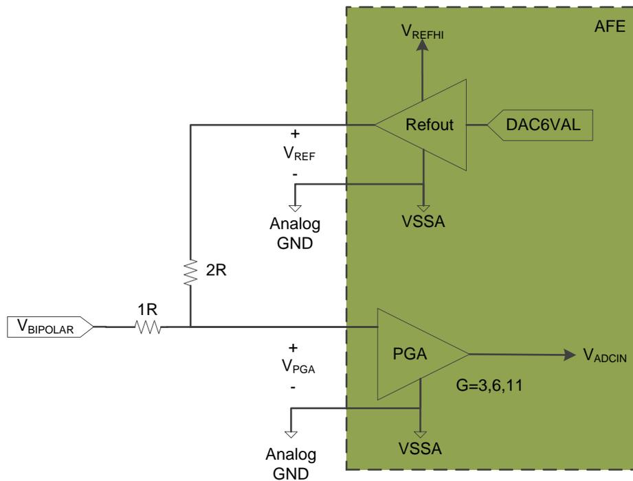
**Figure 12. Using the AFE's Built-In Voltage Reference For Measuring a Bipolar Signal**
