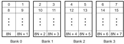
For devices that have more than one memory space (Figure 5-2), an access to bank 0 in one memory space does not interfere with an access to bank 0 in another memory space, and no pipeline stall occurs.
