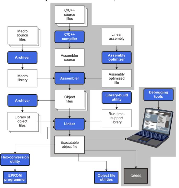
Figure 1-1. TMS320C6000 Software Development Flow
