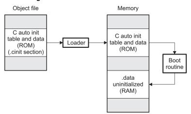
Figure 8-11. Autoinitialization at Run Time
