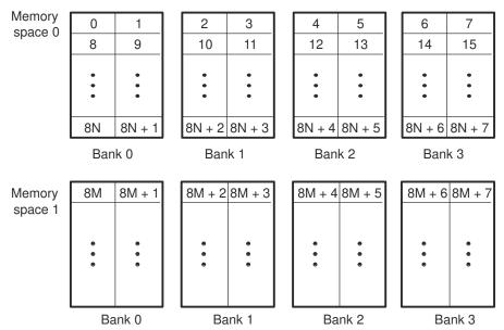
Figure 5-2. 4-Bank Interleaved Memory With Two Memory Spaces
