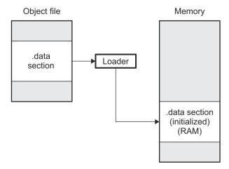
Figure 8-12. Initialization at Load Time
