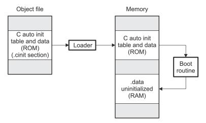
Figure 8-11. Autoinitialization at Run Time
