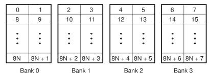
Figure 5-1. 4-Bank Interleaved Memory
