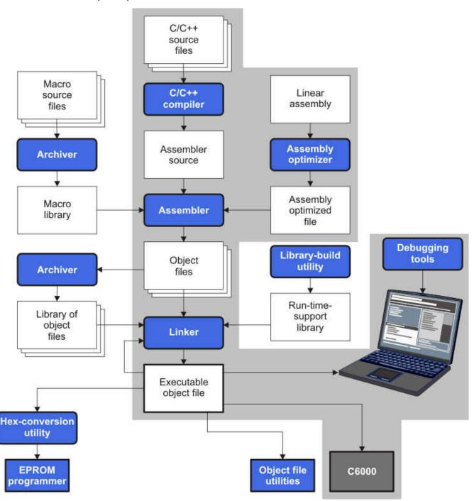
Figure 1-1. TMS320C6000 Software Development Flow
