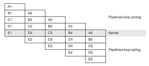
Figure 4-1. Software-Pipelined Loop
