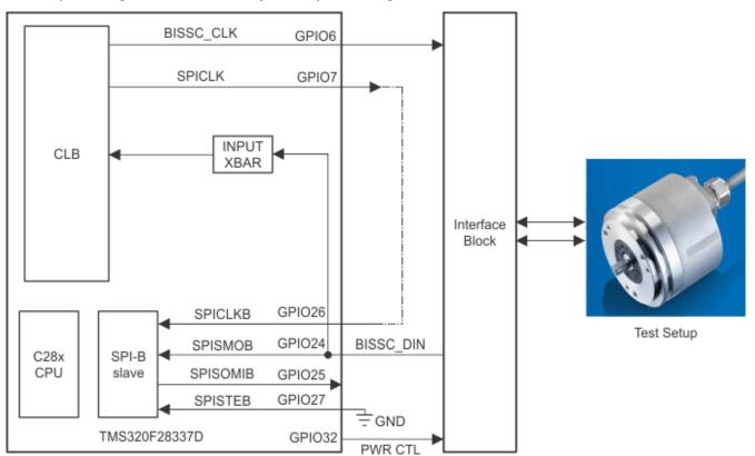
Figure 1-3. BiSS-C Implementation Diagram Inside TMS320F28379D
