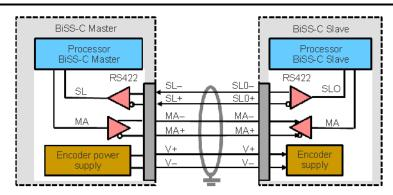
Figure 1-2. BiSS-C Point-to-Point Structure
