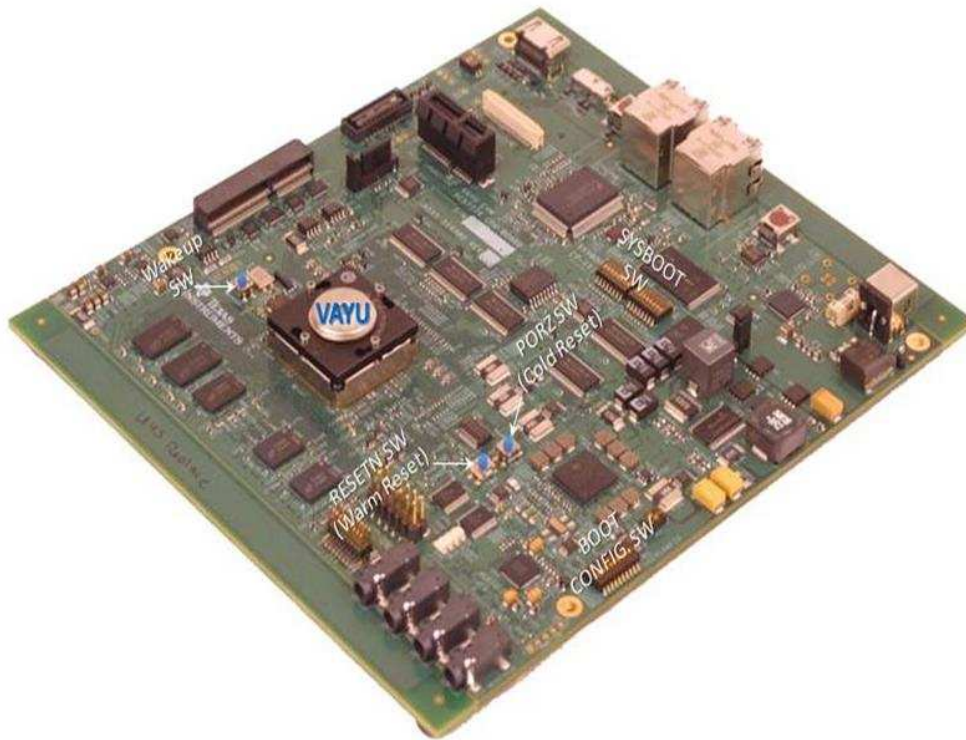
Figure 4. CPU Board Switch and Button Locations (Rev E and earlier)
