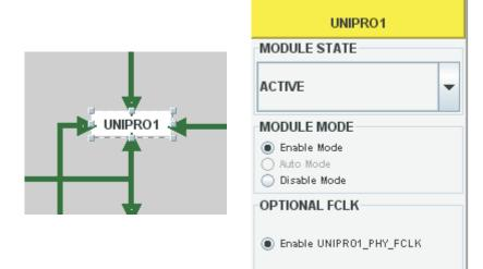
If a module has only ACTIVE/IDLE functionality, the user can switch a module to ACTIVE or IDLE state and only the MODULE STATE drop down menu will be displayed inside the CONTROLLER VIEW.
