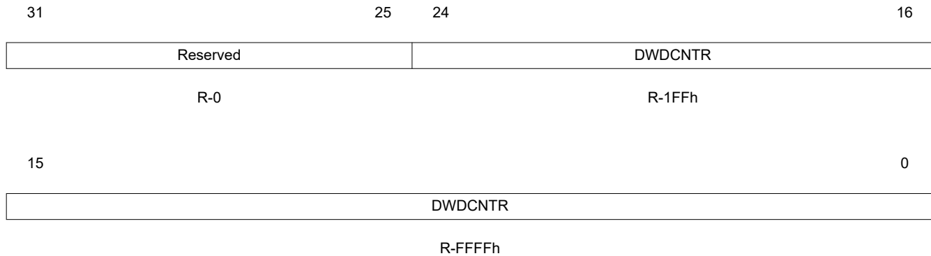
Figure 10-1379. RTI Watchdog Down Counter Register (RTIDWDCNTR) [offset = A0h]
