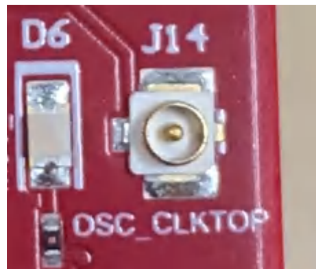
Figure 2-13. OSC Clock Port
