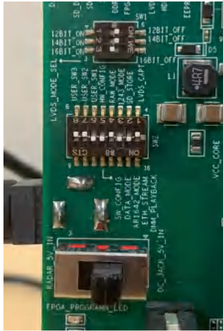
Figure 2-24. DCA1000 Switch Settings
