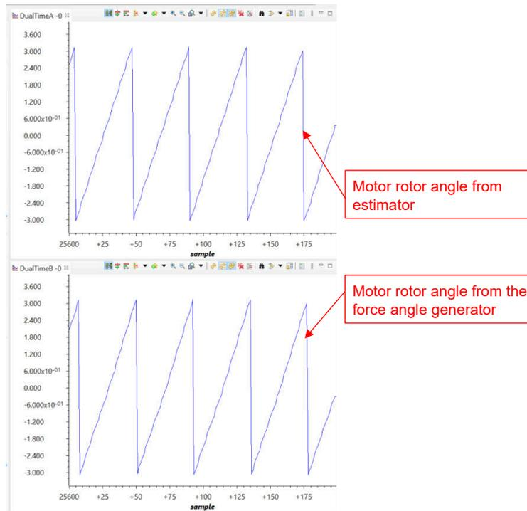
**Figure 3-41. Build Level 2: Motor Rotor Angle Waveforms With Graph Tool**
