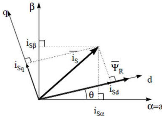
**Figure 2-7. Stator Current Space Vector in The d,q Rotating Reference Frame**
