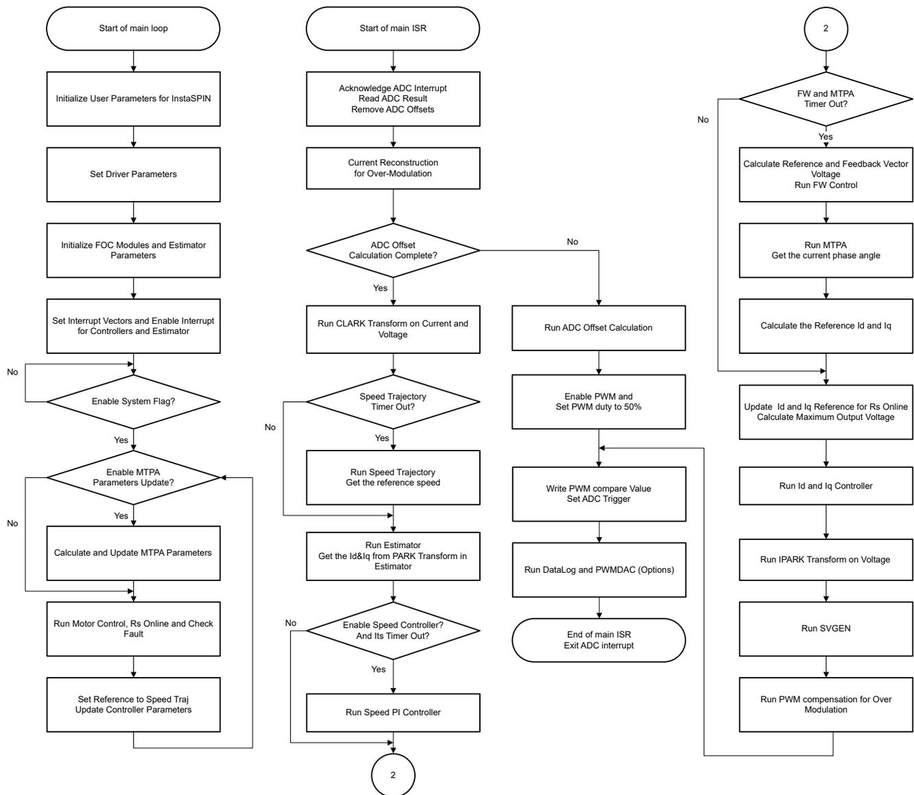
Figure 2-22. Flowchart for an InstaSPIN-FOC Project With FW and MPTA
