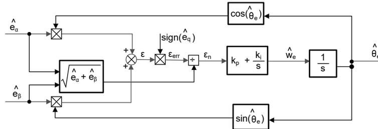
**Figure 2-16. Block Diagram of Phase Locked Loop Position Tracker**
