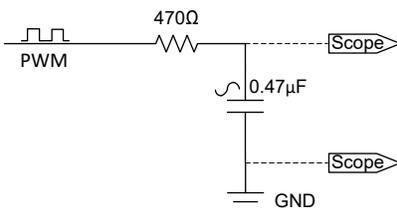
Figure 3-26. External RC Low-Pass Filter Connecting to a PWM Pin of the C2000 MCU
