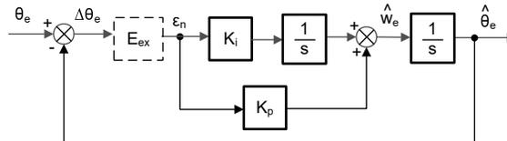
Figure 2-17. Simplified Block Diagram of Phase Locked Loop Position Tracker
