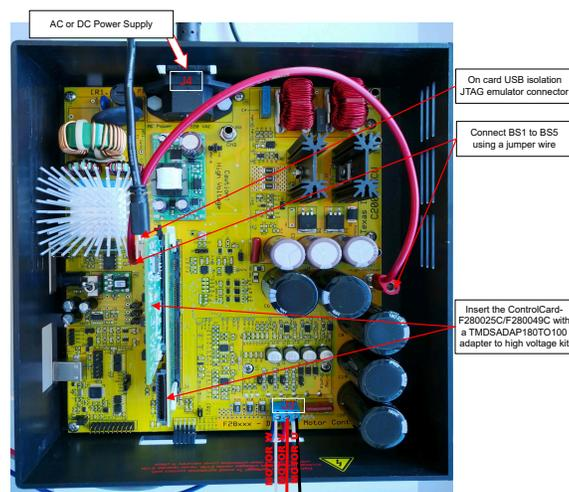
**Figure 3-16. TMDSHVMTRINSPIN Connected to the TMDSCNCD280025C, TMDSCNCD280039C, or TMDSCNCD2800137 with TMDSADAP180TO100**
