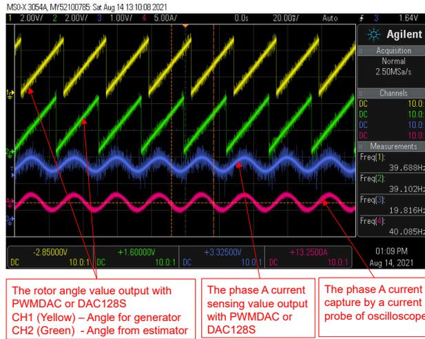
**Figure 3-44. Build Level 3: Motor Rotor Angle and Phase Current Waveforms on Oscilloscope**
