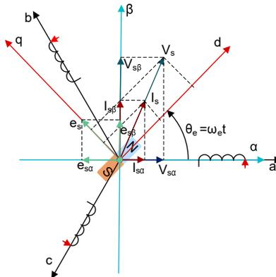
Figure 2-3. Definitions of Coordinate Reference Frames for PMSM Modeling
