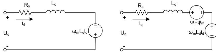
**Figure 2-18. Equivalent Circuit of an IPM Synchronous Motor**
