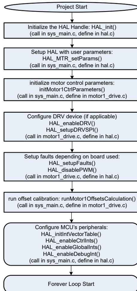
**Figure 4-1. HAL Configuration and Motor Control Setting Block Diagram**
