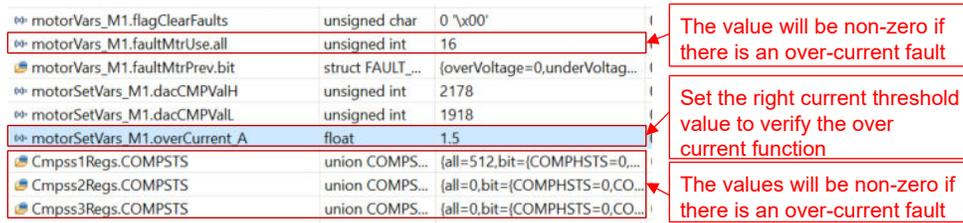
Figure 3-34. Build Level 2: Current Protection Setting
