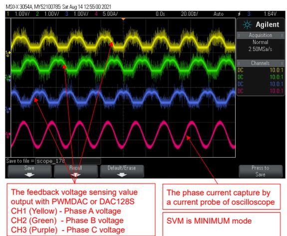
**Figure 3-37. Build Level 2: Motor Phase Voltage Waveforms Using Minimum SVM Mode**
