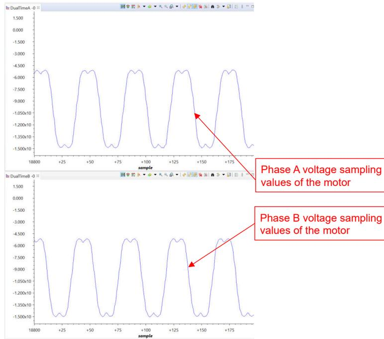
**Figure 3-40. Build Level 2: Motor Phase Voltage Waveforms With Graph Tool**
