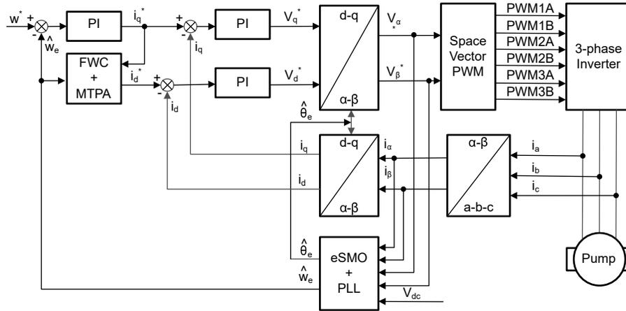
Figure 2-2. Sensorless FOC Structure of an PMSM System
