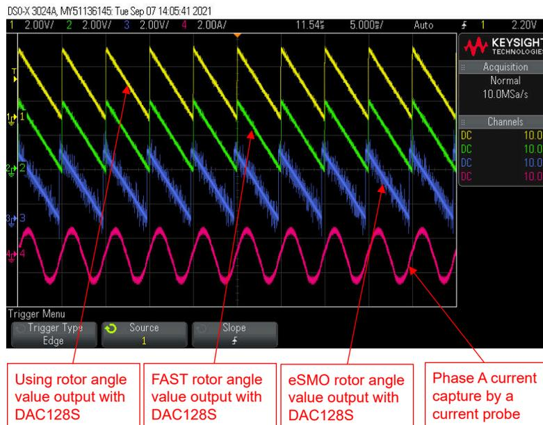
**Figure 3-49. Build Level 4: Rotor Angle With FAST and eSMO, Phase Current Waveforms at Reversal Rotation**
