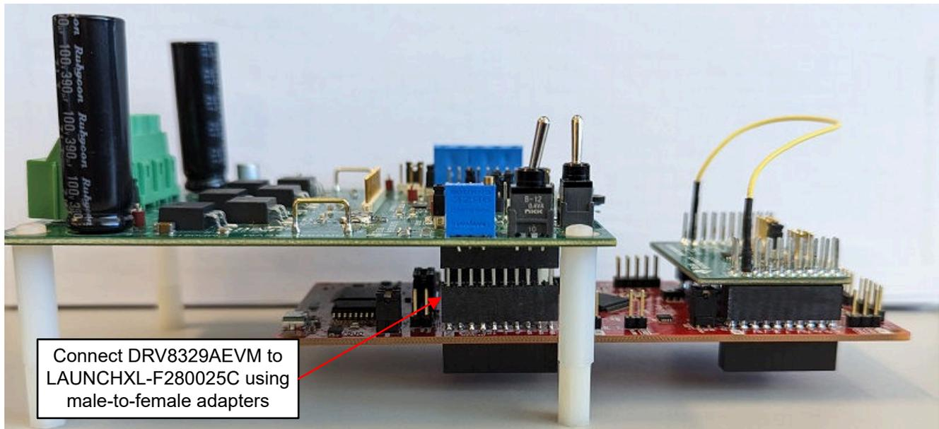
**Figure 3-9. LAUNCHXL-F280025C Connected to the DRV8329AEVM and DAC128S085EVM, Side View**
