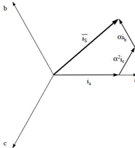
**Figure 2-5. Stator Current Space Vector and its Component in (a,b,c) Frame**
