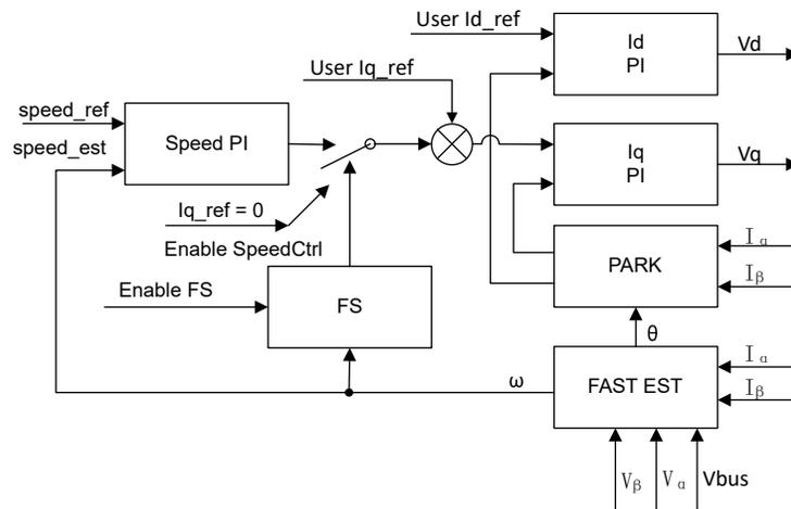
**Figure 2-23. Flying Start Control Block Diagram**
