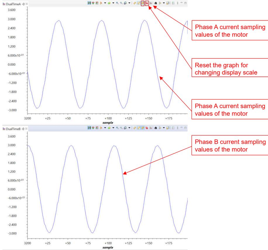
**Figure 3-39. Build Level 2: Motor Phase Current Waveforms With Graph Tool**
