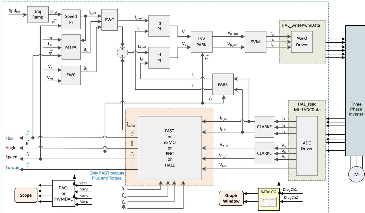
**Figure 3-45. Build Level 4 Software Block Diagram - Speed and Current Close Loop Control**
