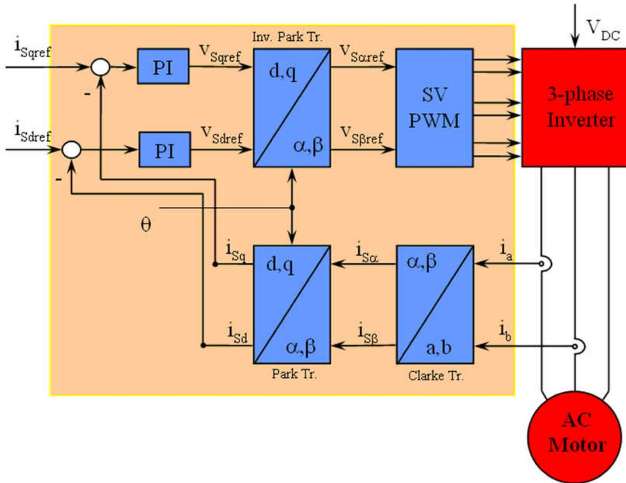
Figure 2-8. Basic Scheme of FOC for AC Motor
