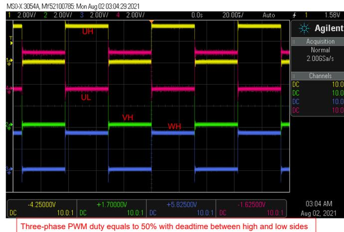
Figure 3-31. Build Level 1: PWM Output Waveforms
