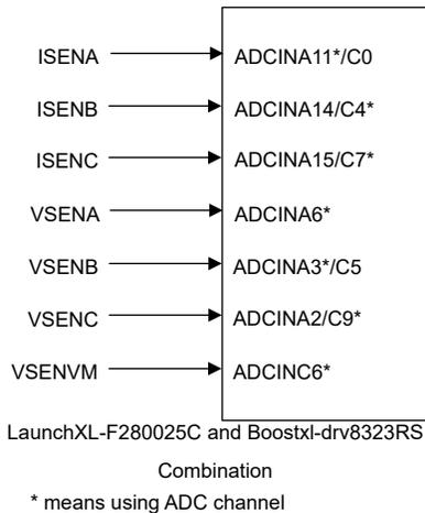
**Figure 4-3. ADC Connection Diagram**
