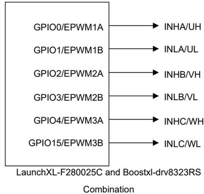
**Figure 4-2. PWM Connection Diagram**
