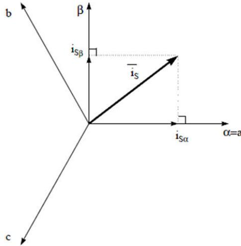
**Figure 2-6. Stator Current Space Vector in the Stationary Reference Frame**
