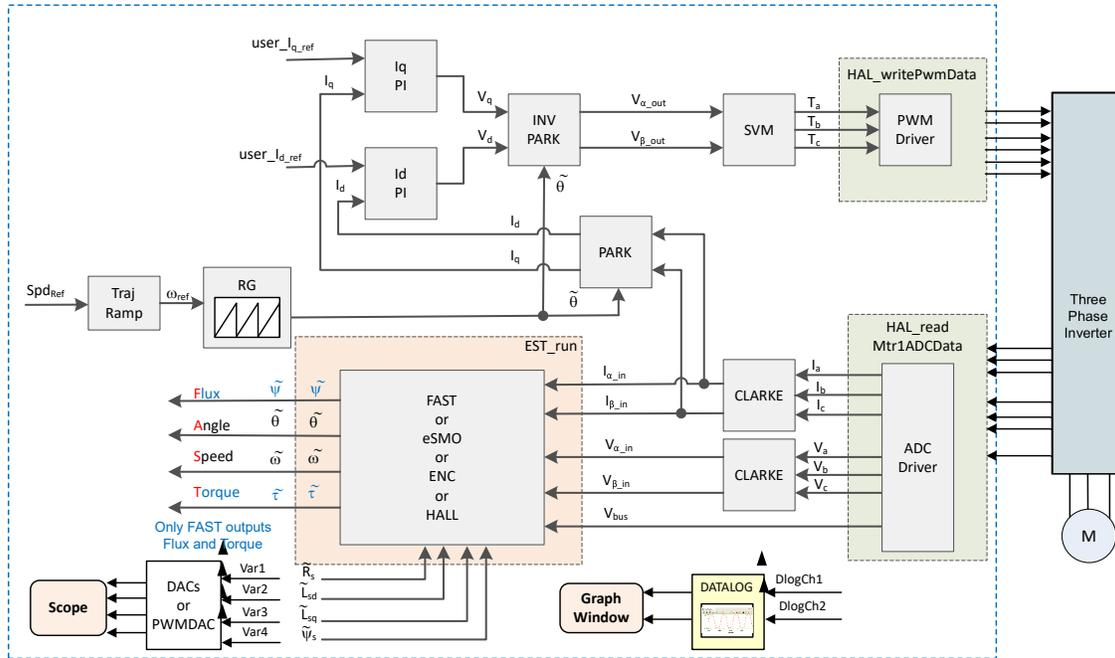
Figure 3-42. Build Level 3 Software Block Diagram - Current Close Loop Control
