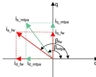
**Figure 2-21. Current Phasor Diagram of an IPMSM During FW and MTPA**
