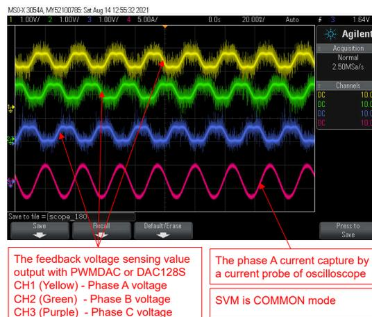
Figure 3-36. Build Level 2: Motor Phase Voltage Waveforms Using Common SVM Mode
