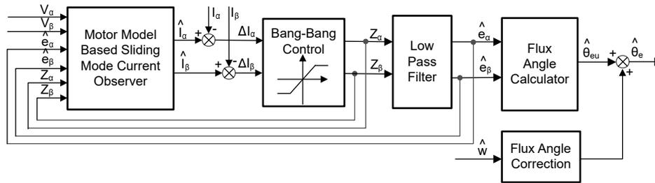
**Figure 2-15. Block Diagram of Traditional Sliding Mode Observer**
