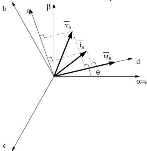
**Figure 2-9. Current, Voltage and Rotor Flux Space Vectors in the  $(d, q)$  Rotating Reference Frame**
