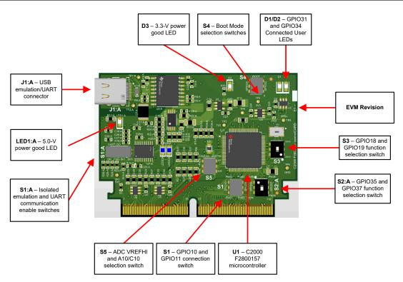
Figure 6-1. Key Components on the controlCARD - Front
