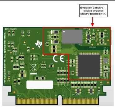
Figure 6-2. Key Components on the controlCARD - Back
