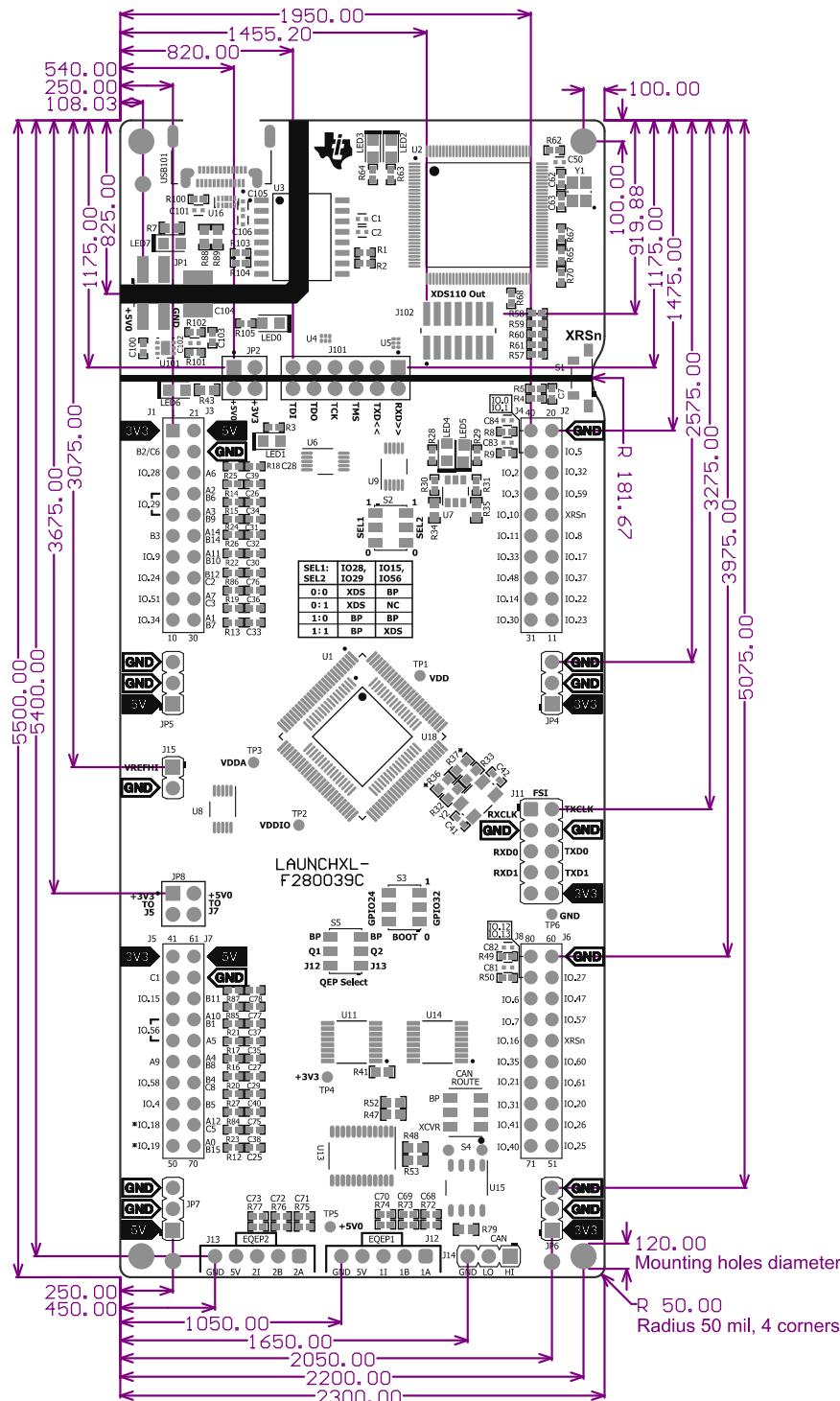
**Figure 4-5. F28003x LaunchPad Dimensions and Component Locations**
