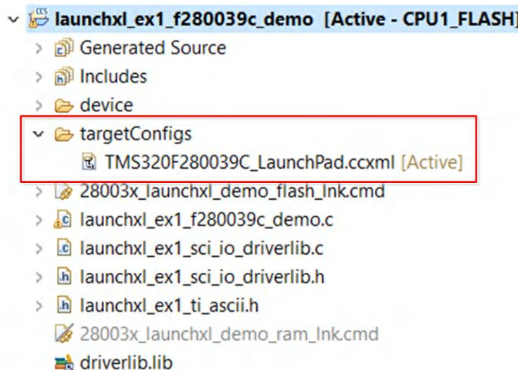
**Figure 5-2. Target Configuration Included in the Demo Project**
