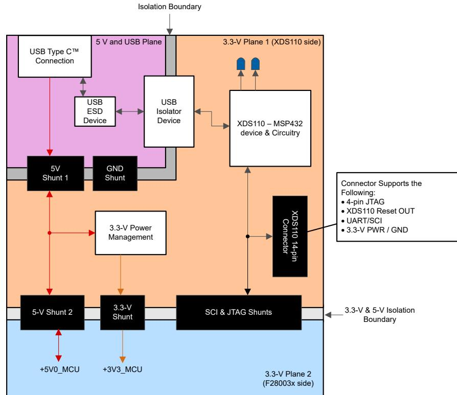
**Figure 3-3. LaunchPad Power Plane Diagram**
