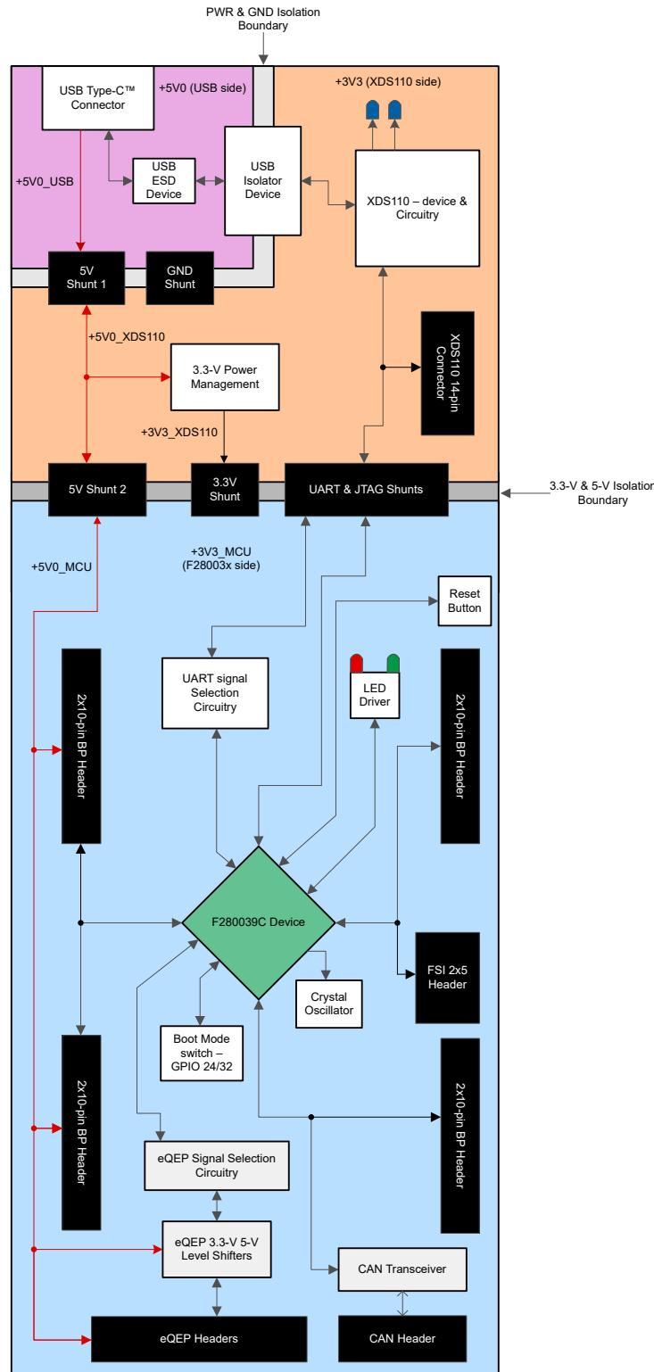
**Figure 3-1. F28003x LaunchPad Development Kit Block Diagram**
