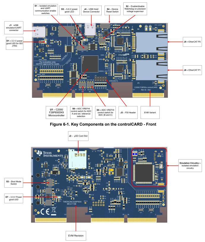
Figure 6-2. Key Components on the controlCARD - Back
