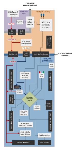
Figure 2-1. F28P55x LaunchPad Development Kit Block Diagram
