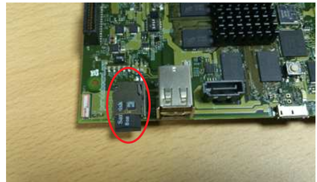
4. Create a micro SD card following the steps as explained in the Software Developers' Guide section 2.2 Prepare SD Card. Insert the micro SD card into the SD card slot, with Micro SD card label facing up.
