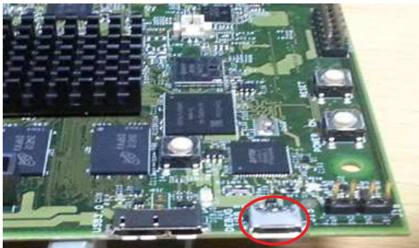
5. Connect a Debug USB via micro-USB connector via micro USB port (J15). Connect the other end of the serial cable to a PC. This step is optional. This step enables viewing of console messages on a PC terminal and changing some of the default parameters on the board.
