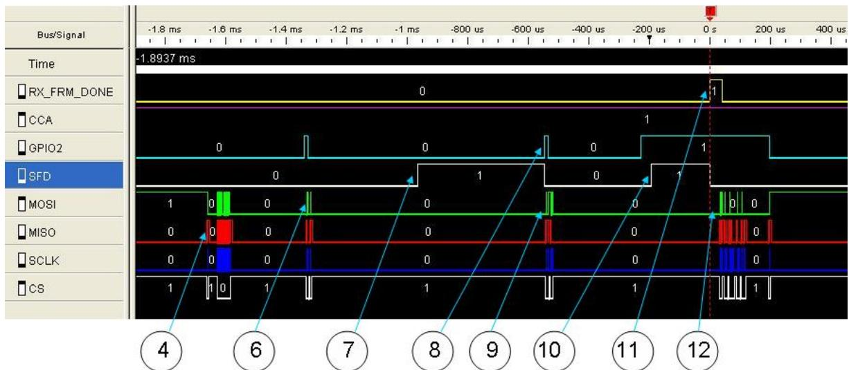
Figure 15 Capture of packet transmission scenario using a logic analyzer
