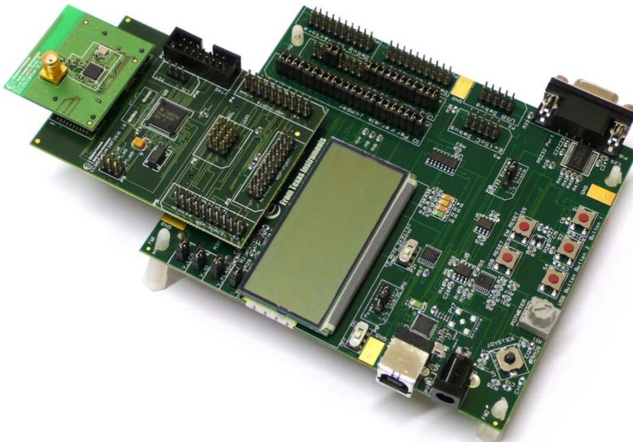
Figure 1 SmartRF05EB/CCMSP2618/CC2520EM
