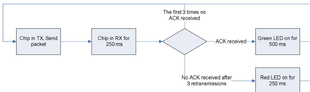
**Figure 3 Cycle for master node**
