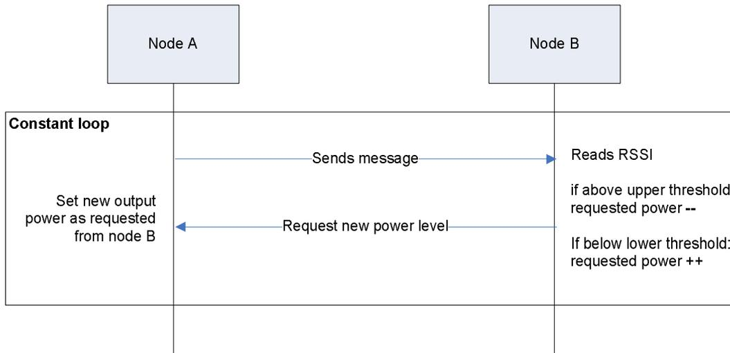
**Figure 5 Sequence diagram of the adaptive power adjustment**
