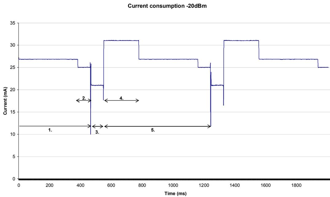
**Figure 12 Slave node sending 2 ACK's**
