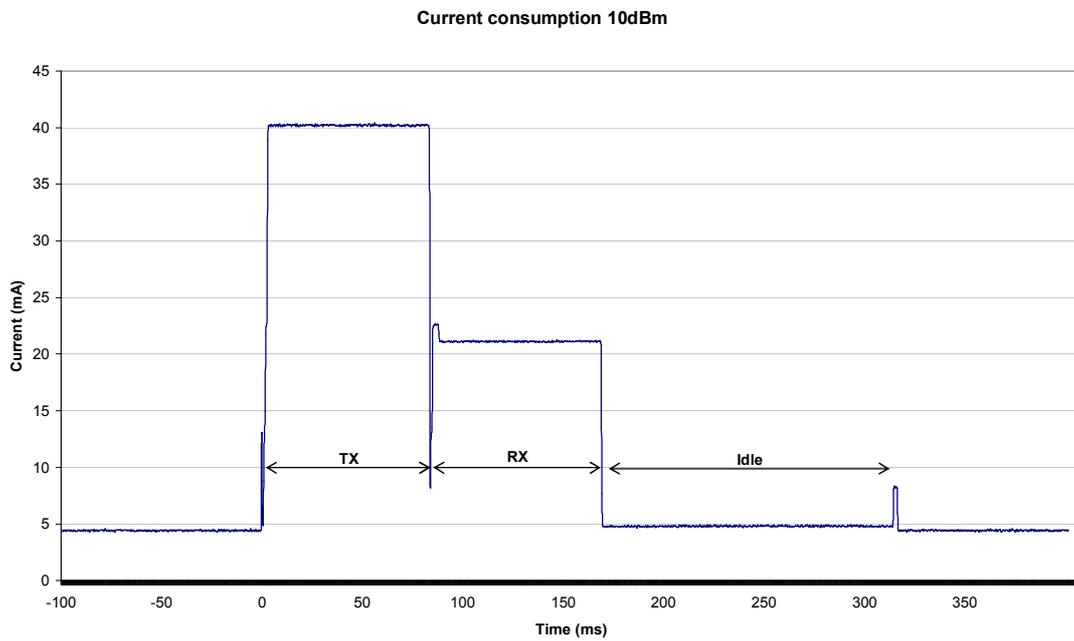
**Figure 9 Current consumption for CC1110 Mini DK at 10dBm output power**
