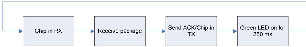
**Figure 4 Cycle for slave node**
