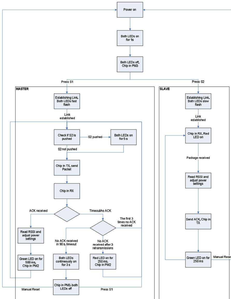
**Figure 1 Flow chart for the Simple Link Application**
