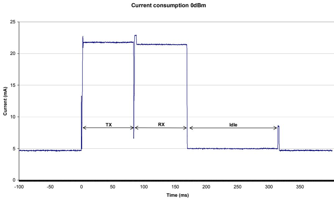
**Figure 8 Current consumption for CC1110 Mini DK at 0dBm output power**
