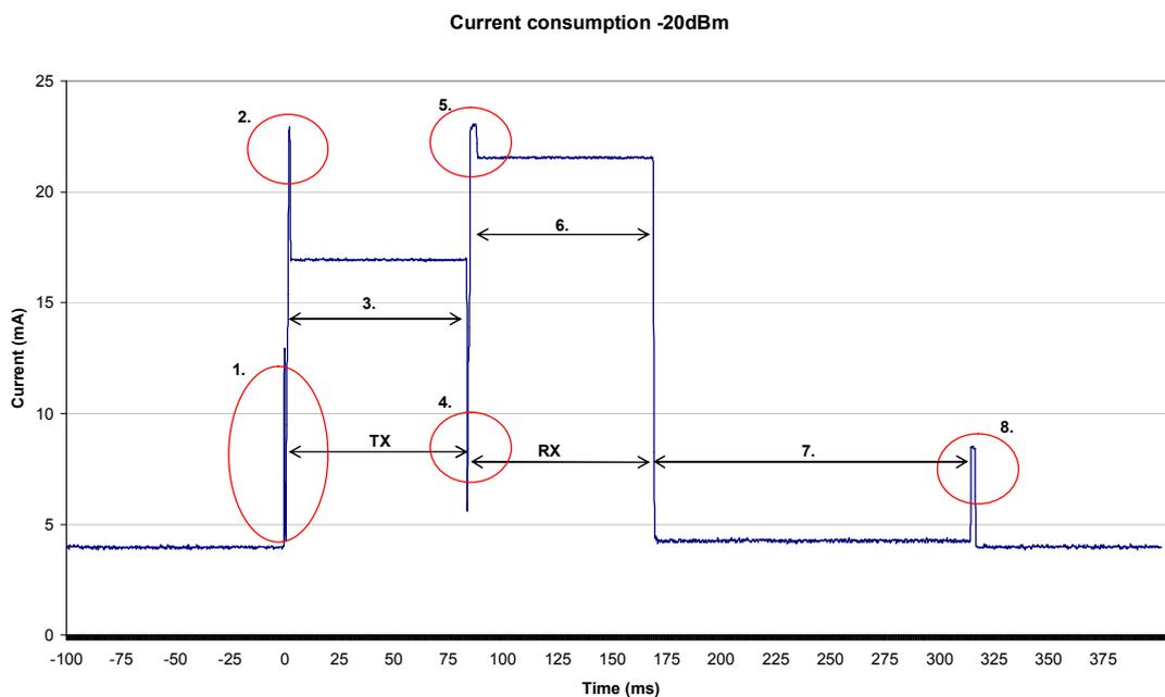
**Figure 7 Current consumption for CC1110 Mini DK at -20dBm output power**
