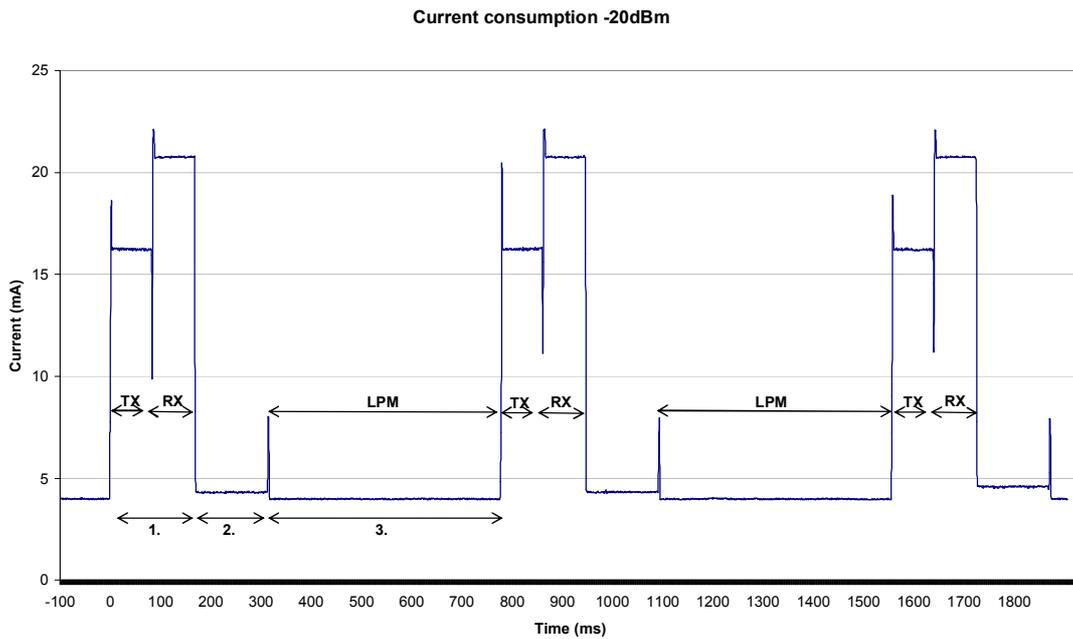
**Figure 10 Time plot of three TX/RX cycles**
