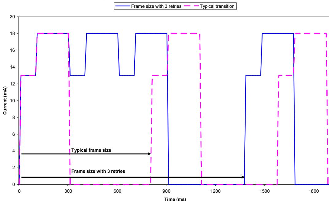
**Figure 6 Different frame time dependent of retries**
