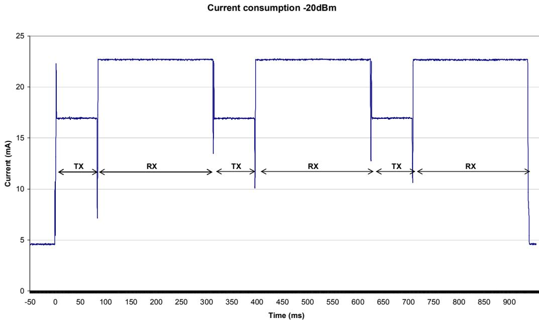
**Figure 11 Current consumption for CC1110 Mini DK at -20dBm output power and 3 retransmits**
