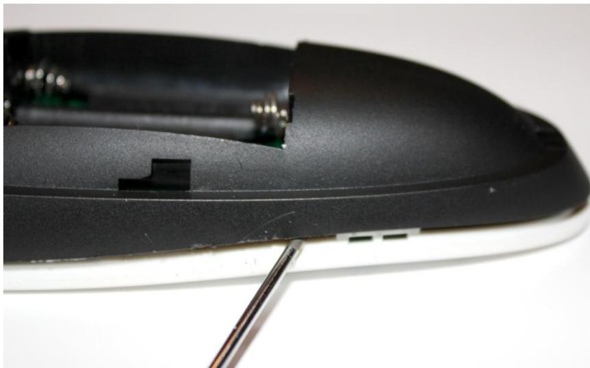
**Figure 7-2: Opening the remote control**
