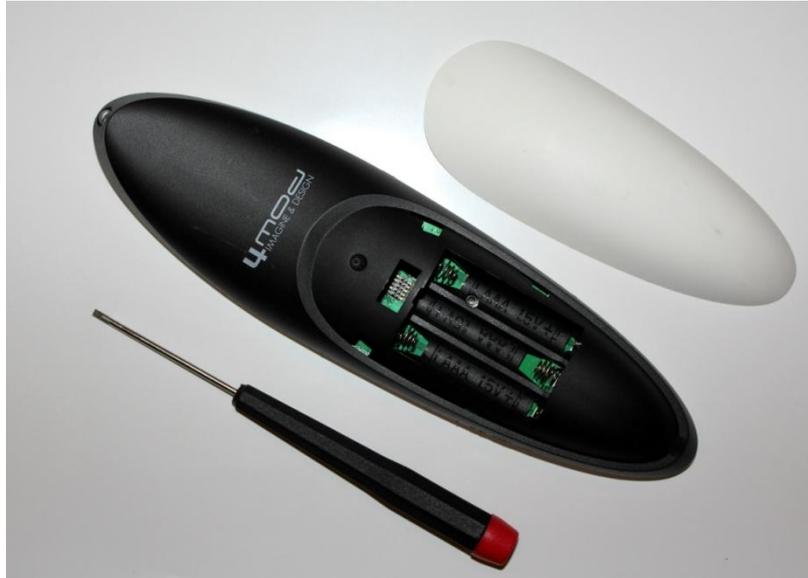
**Figure 7-1: Tools for opening the remote**
