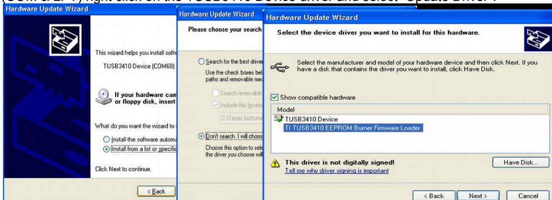
**Figure 8-2: Installing the EEPROM burner driver**
