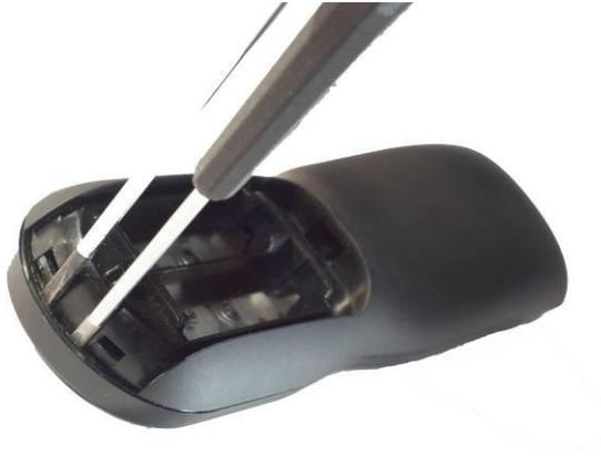
**Figure 7-3: Opening the remote control, step one**
