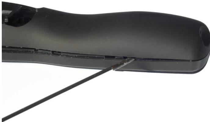
**Figure 7-4: Opening the remote control, step two**
