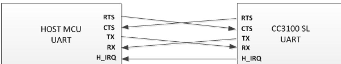
**Figure D-12. Typical 5-Wire UART Configuration**
