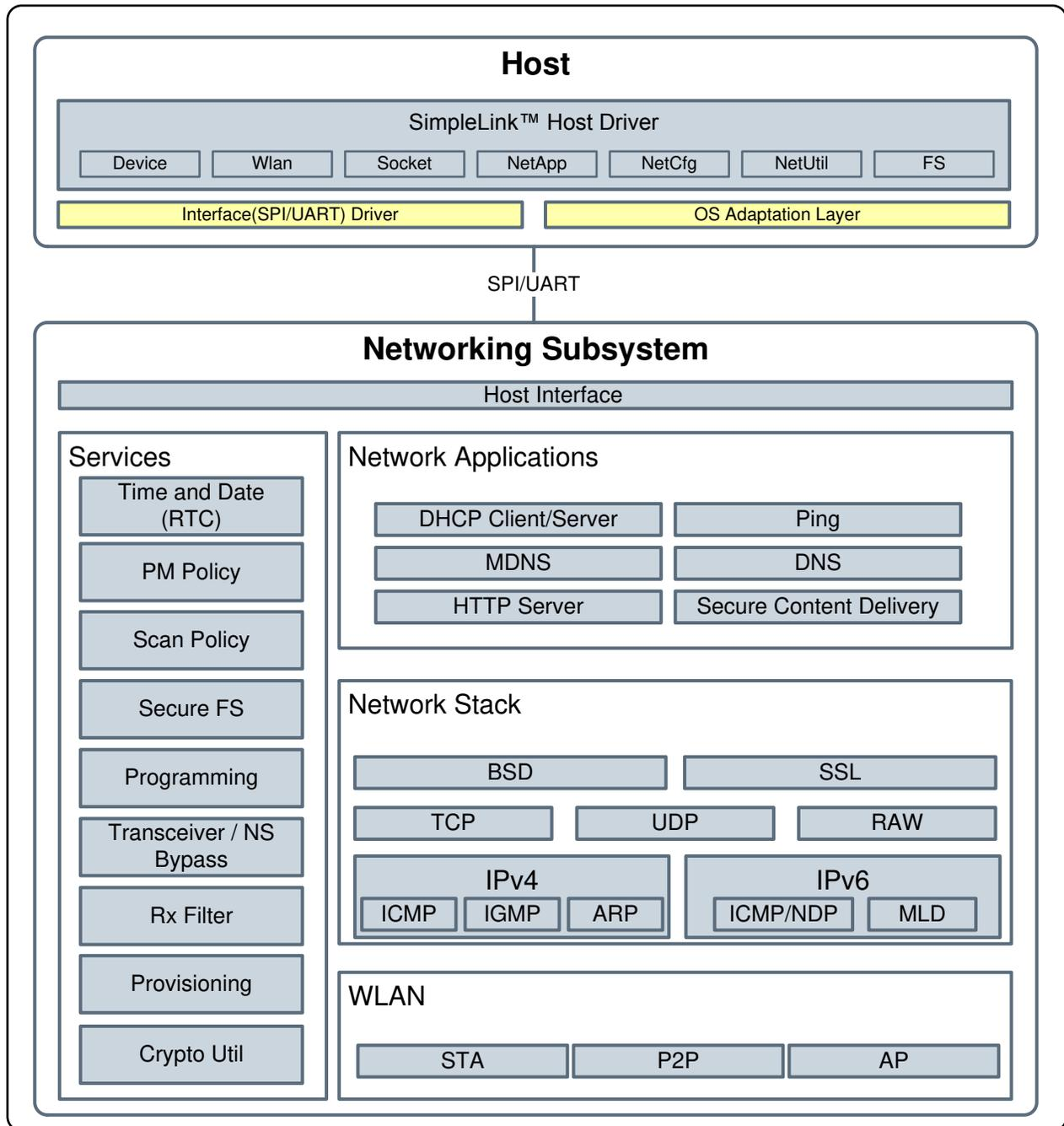
Figure 1-2. Networking Subsystem Block Diagram
