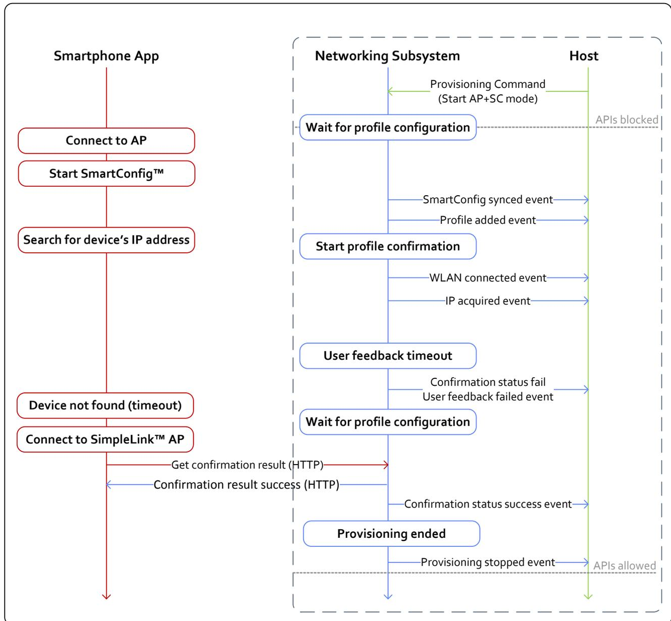
Figure 16-5. Successful SmartConfig Provisioning With AP Fallback
