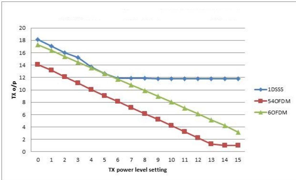
Figure 4-1. Tx Output Power vs Tx Power Settings
