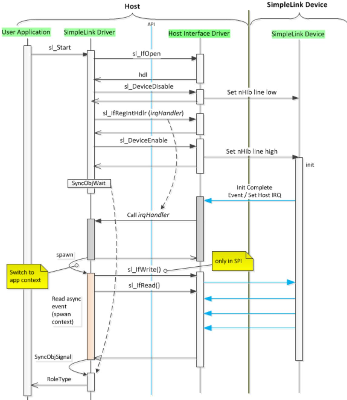
Figure D-5. SPI Initialization Flow
