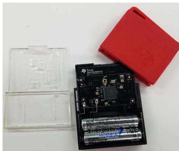
**Figure 11. Replacing the Batteries**
