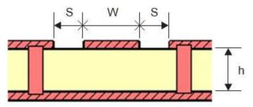
Figure 12. Coplanar Waveguide (Cross Section) With GND and Via Stitching
