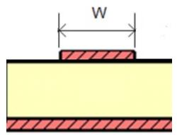
Figure 11. Microstrip Transmission Line
