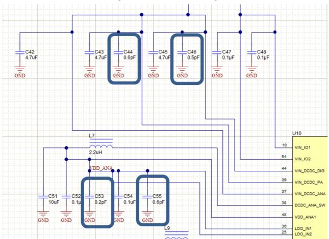
Figure 20. 5-GHz DC/DC Filtering
