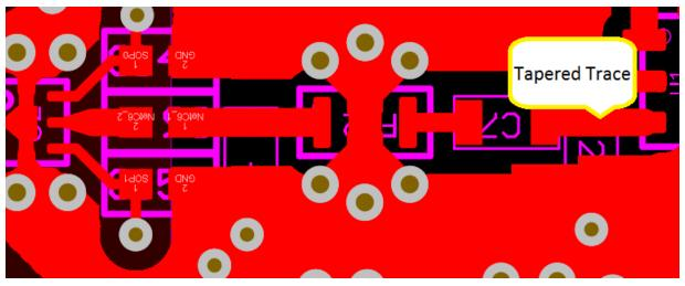
Figure 14. Filleting and Tapering of the Line
