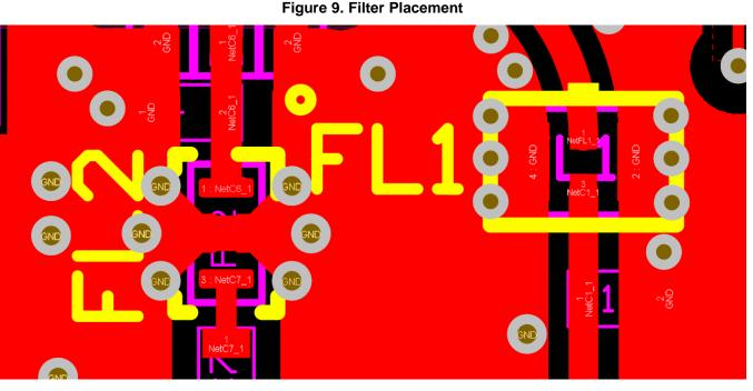
The RF filter must be placed close to the device pin, between the antenna and the device. The RF filter should have a good ground connection to the L2 ground plane. TI recommends adding at least two ground vias near the ground pins to ensure good RF grounding.
