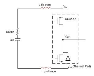
Table 14 describes the maximum allowable trace inductance for the three DC/DC converters.
