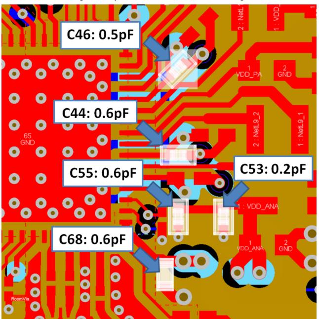
Figure 22. Layout for 5-GHz DC/DC and SOP2 Filtering
