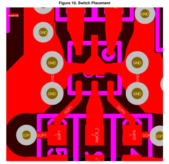
The RF switch should have a good ground connection to the L2 ground plane. TI recommends adding at least two ground vias on both sides ground pad to ensure good RF grounding. Care must be taken in routing the path to the control pins to ensure minimal noise on line
