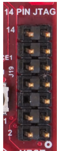
Figure 2-21. 14-Pin JTAG Connector
