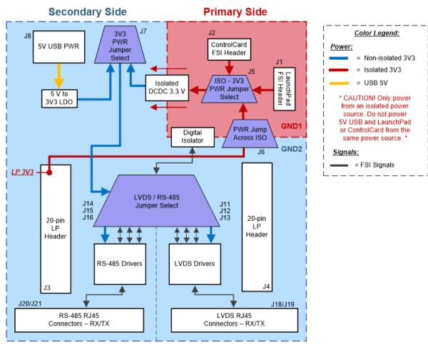
Figure 9. Power Domains Block Diagram
