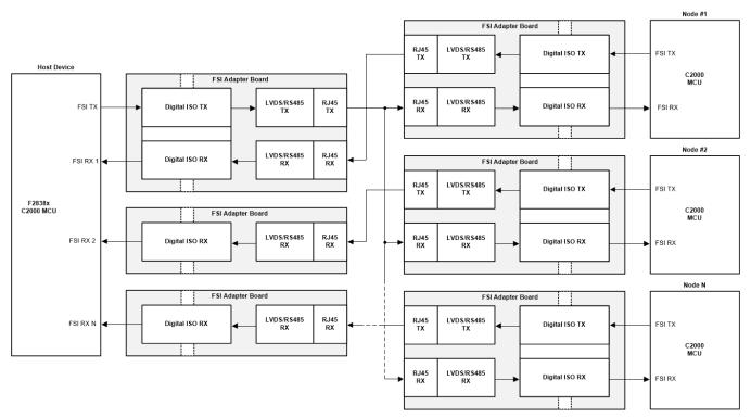
Figure 17. FSI Star Connection Block Diagram
