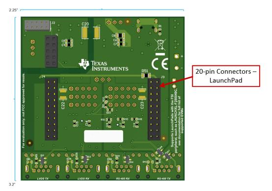
Figure 3. FSI Adapter Board - Back Side Hardware
