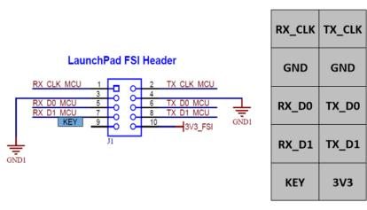
Figure 5. J1 LaunchPad FSI Connector Signals
