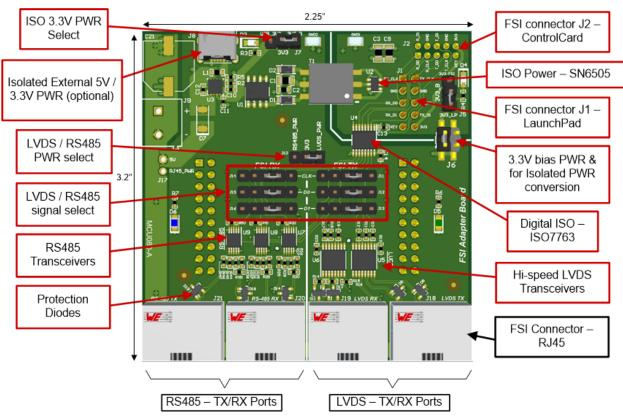
Figure 2. FSI Adapter Board - Front Side Hardware
