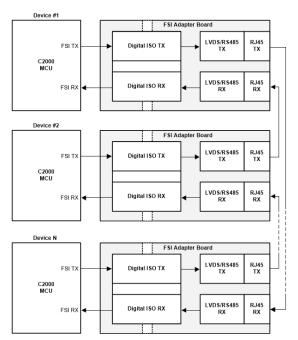
Figure 16. FSI Daisy-chain Block Diagram
