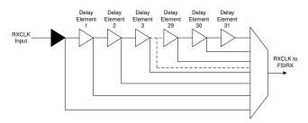
Figure 15. Delay Line Control Circuit
