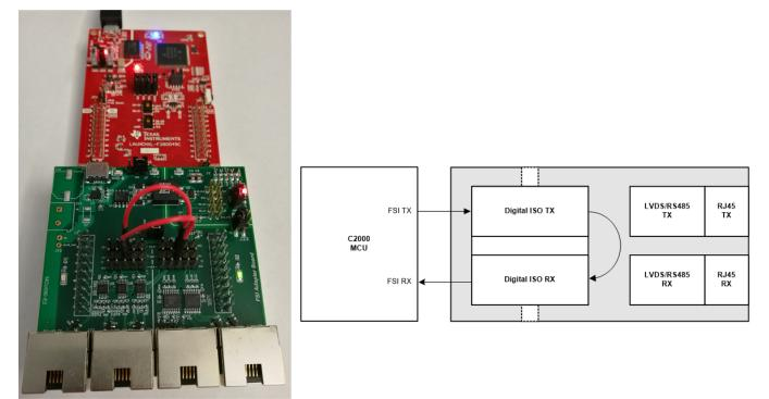
Figure 13. ISO No-Transceiver Loopback Hardware Setup
