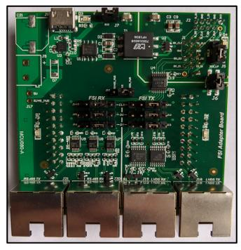
Figure 1. FSI Adapter Board
