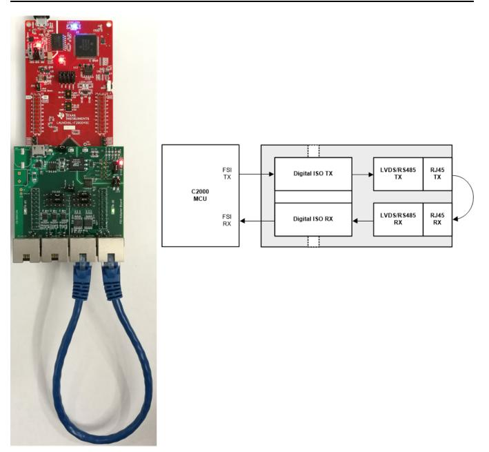
Figure 10. CAT5 External Loopback Hardware Setup
