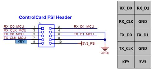
Figure 7. J2 controlCARD FSI Header Signals
