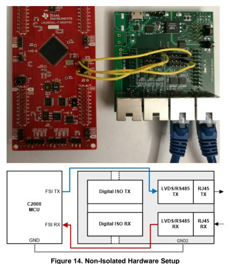
**NOTE:** Only the secondary side of the Adapter Board must be powered for the implementation described in Section 5.2. Proper ground connections from the target device to GND2 should be made.
