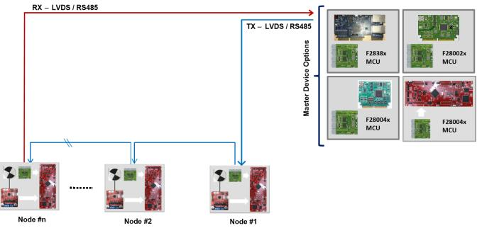
Figure 18. Distributed Multi-axis Servo Example
