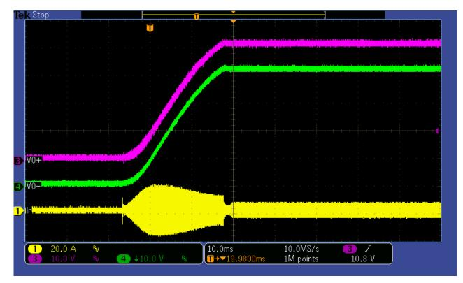
The photo below shows the output voltage startup waveform after the application of 220VAC and loaded to 6A. (CH1: resonant current, CH3: +42V output voltage, CH4: -42V output voltage)
