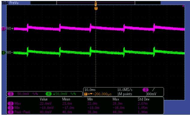
The output ripple voltage is shown in the figure below. The image was taken with the ±42V output loaded to 0A and the input voltage set to 220VAC. (CH3: +42V output in AC coupling, CH4: -42V output in AC coupling)
