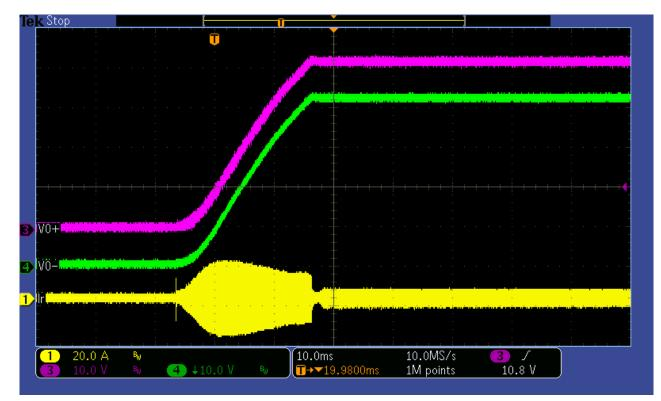
The photo below shows the output voltage startup waveform after the application of 110VAC and loaded to 6A. (CH1: resonant current, CH3: +42V output voltage, CH4: -42V output voltage)
