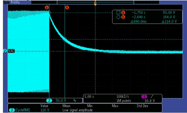
The photo below shows the input voltage waveform after the 240VAC disconnects at no load conditions. (CH2: Input voltage)
