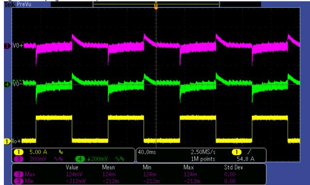
The photo below shows the  $\pm$ 42V output voltage when the load current is stepped between 0A and 6A with an input voltage of 220VAC. (CH1: +42V output current, CH3: +42V output voltage in AC coupling, CH4: -42V output voltage in AC coupling and inverted)
