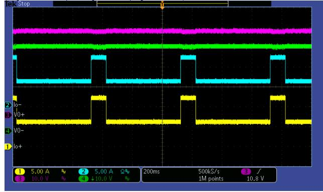
The photo below shows the ±42V output voltage when the load current is stepped between 6A and 12A with an input voltage of 220VAC. (CH1: +42V output current, CH2: -42V output current, CH3: +42V output voltage in AC coupling, CH4: -42V output voltage in AC coupling and inverted)
