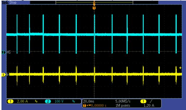
The photo below shows the switch node voltage (Q601 Vds) and resonant current waveforms at full load. The input voltage is 220VAC and the  $\pm$ 42V output is loaded to 6A. (CH1: resonant current; CH2: Q601Vds)
