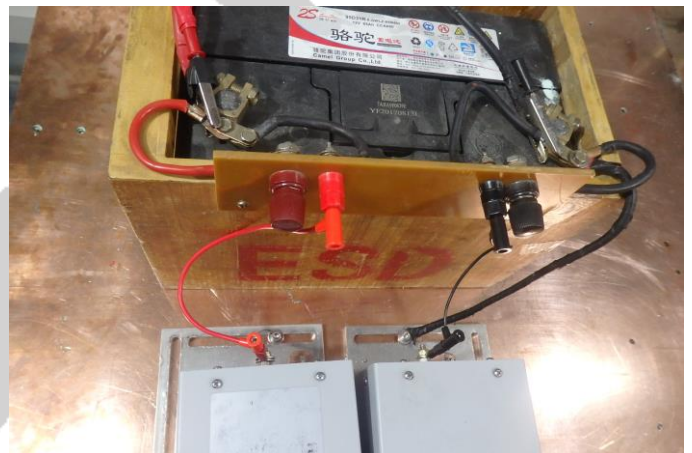
Picture for battery & LISN grounding
