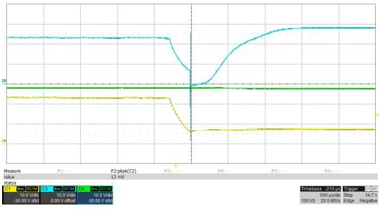
CH1 (YEL): INPUT (J2), 10 V/div CH4 (GRN): BATTERY (J3), 10 V/div CH3 (BLU): OUTPUT (J1), 10 V/div 500 usec/div
