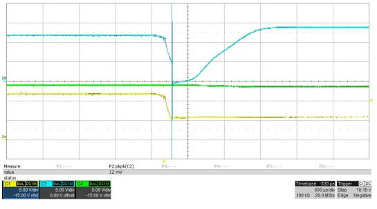
CH1 (YEL): INPUT (J2), 5 V/div CH4 (GRN): BATTERY (J3), 5 V/div CH3 (BLU): OUTPUT (J1), 5 V/div 500 usec/div
