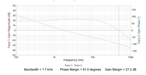
3.3 Bode Plot – LM5176 – 22 V Input, 28 V Output/0.5 A
