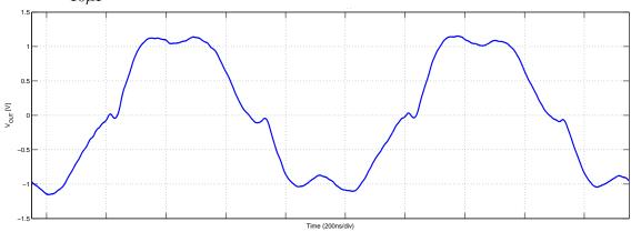
Figure 6.2: Measured Output Signal, Sine Input,  $f_{IN}=5MHz,\,V_{IN}=20\mu V_{PP},\,C_{AC-GAIN}=10\mu F$
